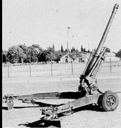
155 mm howitzer L33 X1415 CITEFA Model 77 in firing position with barrel at maximum elevation
