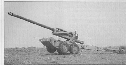
Argentina's 155 mm/45 calibre Long Range Artillery Cannon is expected to have a maximum range of 39 000 m (CITEFA)
