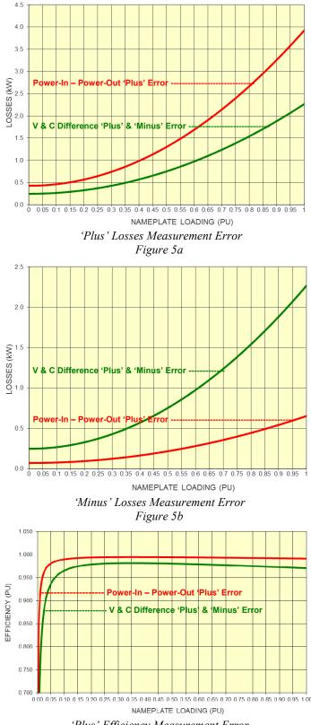
Plus' Efficiency Measurement Error Figure 6a
