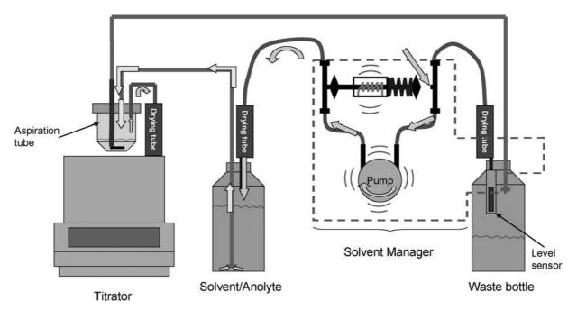
Step 3: The pump direction is switched by activation of the magnetic valve and subsequently fresh solvent is pumped into the titration cell by applying over pressure of dry air.
