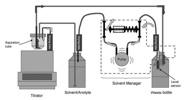
Step 2: The Anolyte is drained into the waste bottle by applying vacuum.
