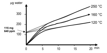
The determination was carried out for a period of 20 minutes (max. time) with the drying oven set to 120  $^{\circ}$ C, 160  $^{\circ}$ C and 250  $^{\circ}$ C. The following results were obtained:
