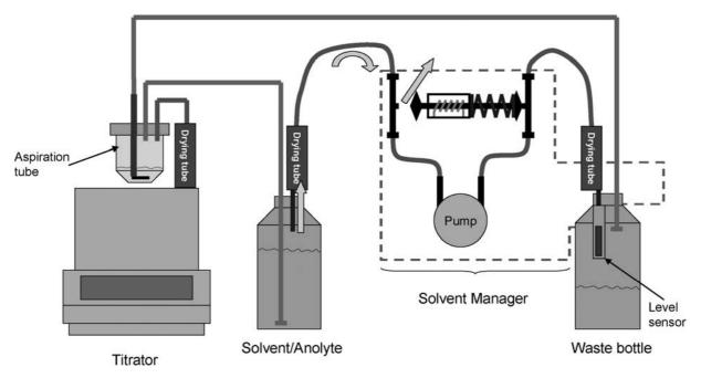
Step 4: After a predefined time or by manual interaction the pressure within the solvent/anolyte bottle is relieved by switching the magnetic valce into the initial position.
