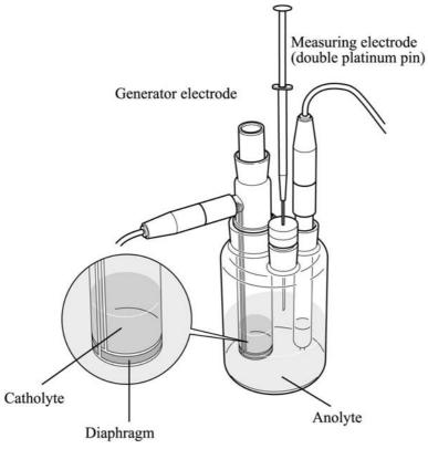
\* The terms "generator electrode" and "measuring electrode" mean an arrangement of two electrodes (anode and cathode) to form an electrolytic cell.
