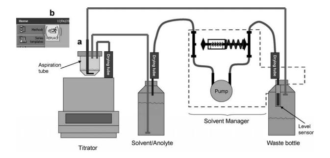
Step 1a: Put the draining and reagent refill tube into the coulometric titration cell.
