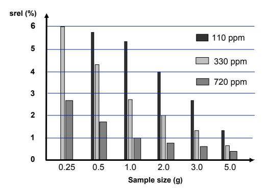
In both cases, with decreasing sample size the relative standard deviation srel becomes worse. Therefore, it is necessary to use the optimum sample size in order to achieve precise results. A good repeatability is achieved the sample size is increased particularly for low water content values.
