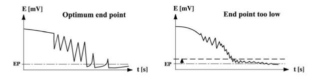
The consequences of choosing a too low end point value are illustrated in the figures above: On the right side, the titration curve is more or less flat towards the end; this results in an illdefined titration end point, which will lead to long titration times and to low precision.
