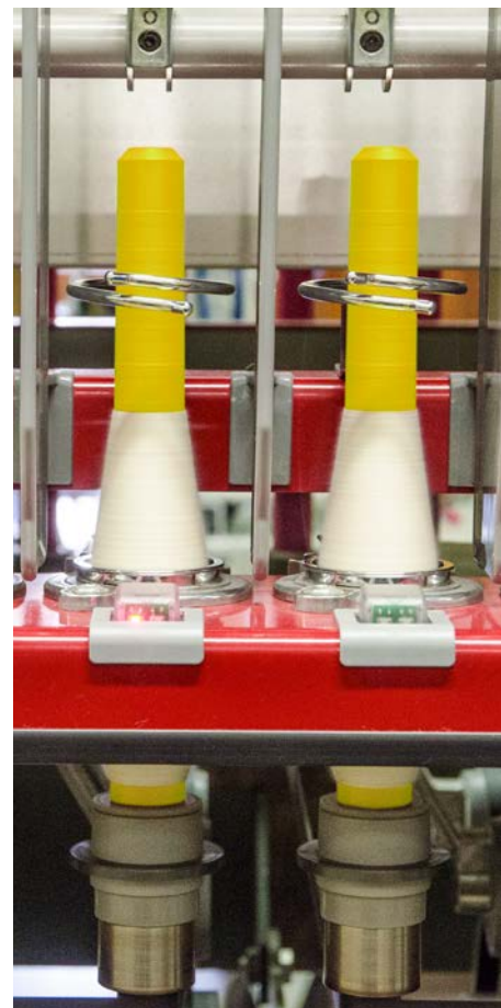
The LED display at the section and at the individual spinning positions leads the operator directly to the affected spindle.
