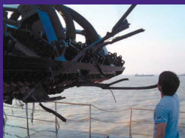
The 'Wild Dragon ® ' draghead seemed to gobble up anything that crossed its path, even a sunken buoy. It cost some teeth but barely dented the rest.
