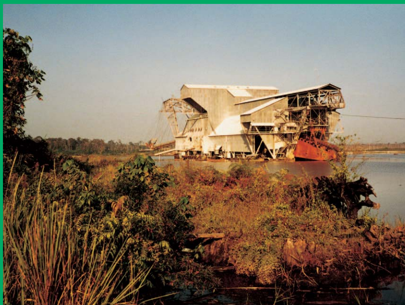
The MARAS, one of the six bucket dredgers IHC delivered in 1947
