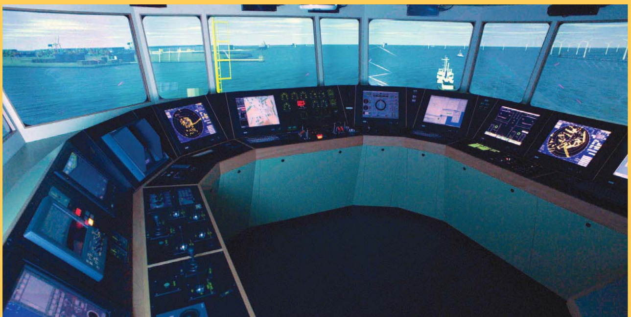
The Zeebrugge simulator with outside view projection. IHC Systems delivered and set up the dredging part of the simulator.
