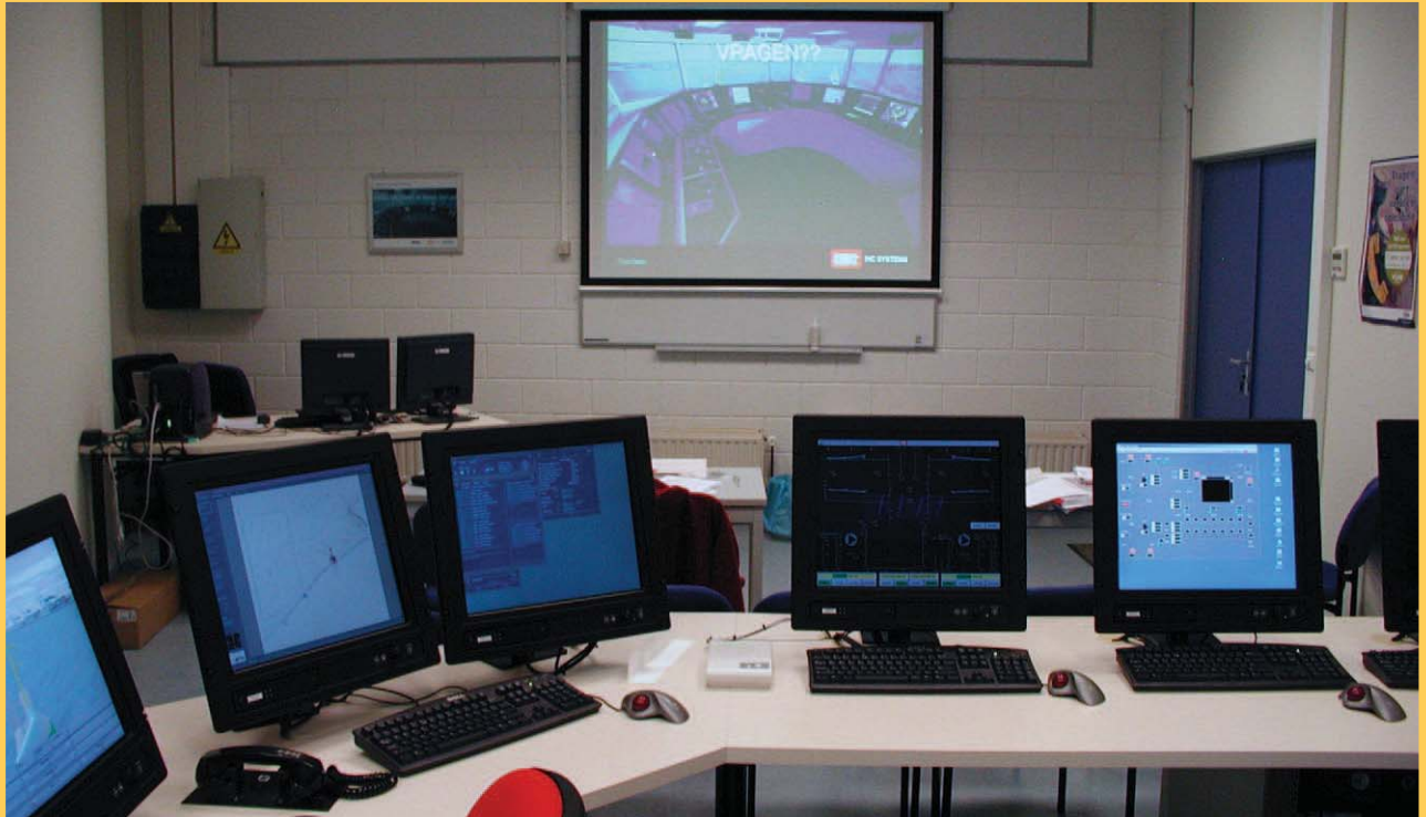
Instructor's desk/debriefing station. From his station, the instructor can send all kinds of data: position, speed and extreme weather conditions, as well as specific data that can influence the dredging process. The debriefing station (background) is where each simulated situation can be evaluated. A bird's eye view projection on the wall screen is possible in some cases.
