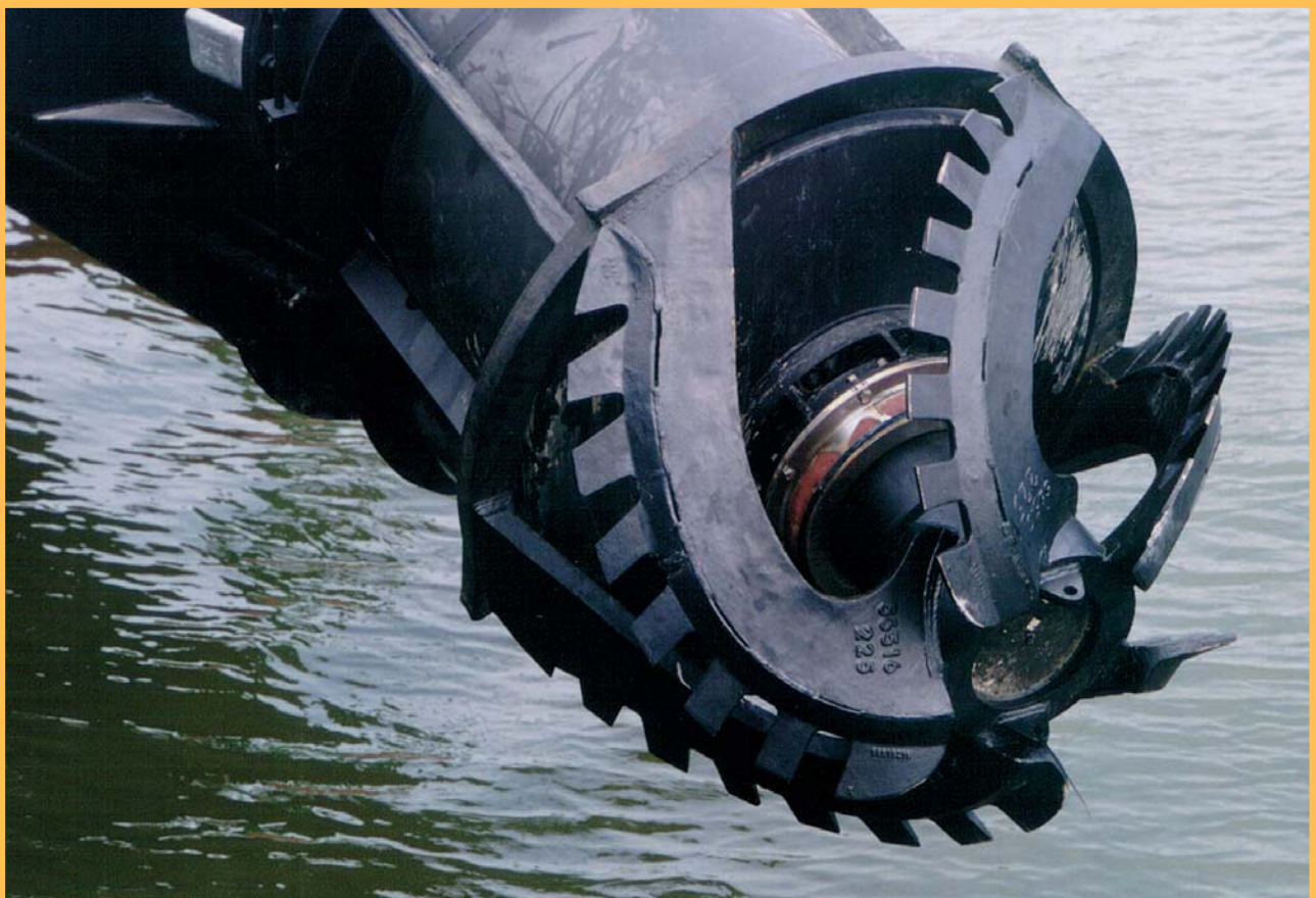
Cutter with cutting edges
