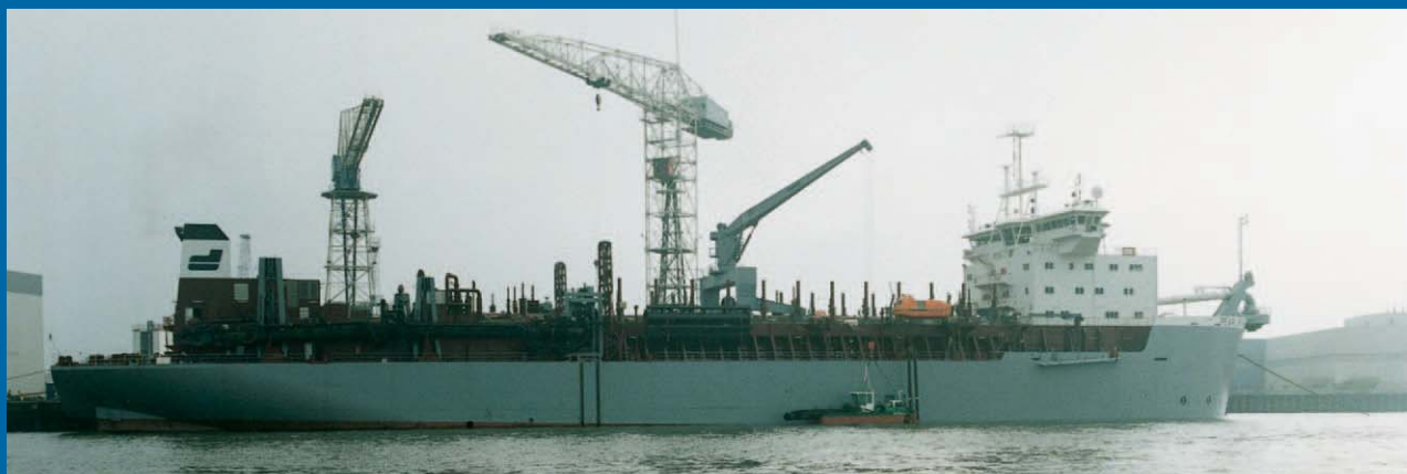
Before: 144m - 17,000m 3 - max. dredging depth 50m
