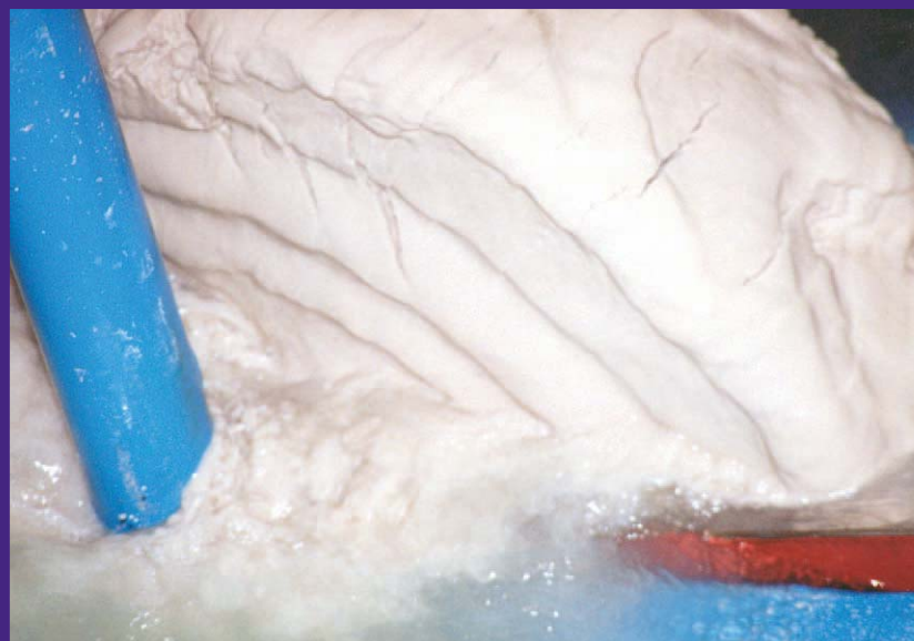
Laboratory test of 'Wild Dragon®' cutting compacted fine sand. After cutting, the sand comes up like a sausage, still needing of (lots of) water before there can be any hope of moving it hydraulically.
