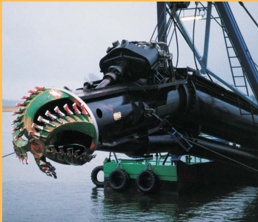
The basic cutter skeleton consists of a hub, a ring and several curved arms linking them together. On the front side of the cutter arms, adapters with teeth or replaceable cutting edges are fitted that do the actual cutting work.
