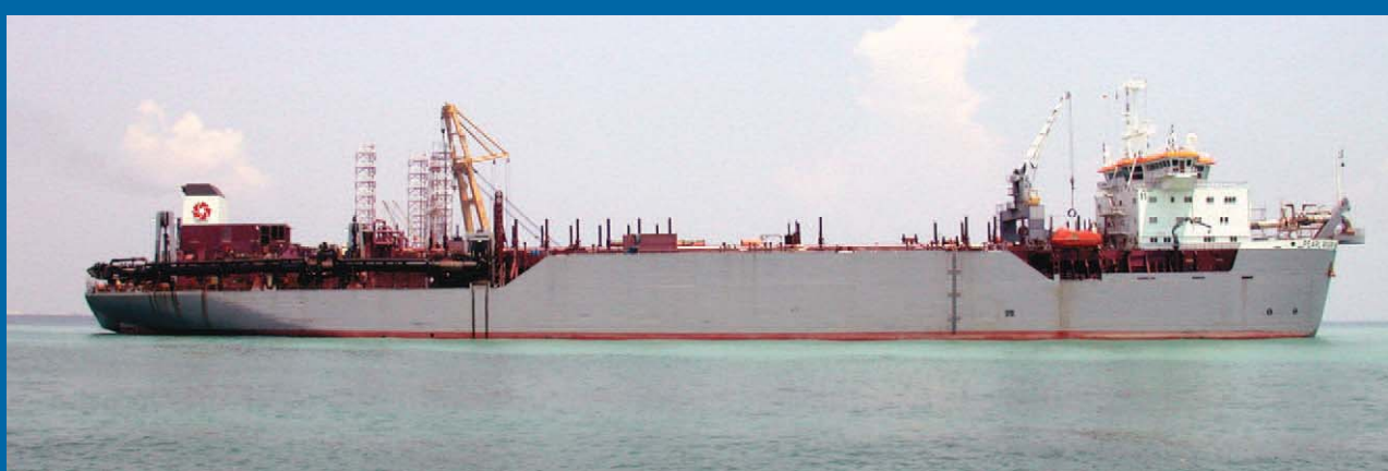
After: 181.80m - 24,124m 3 - max. dredging depth 122m
