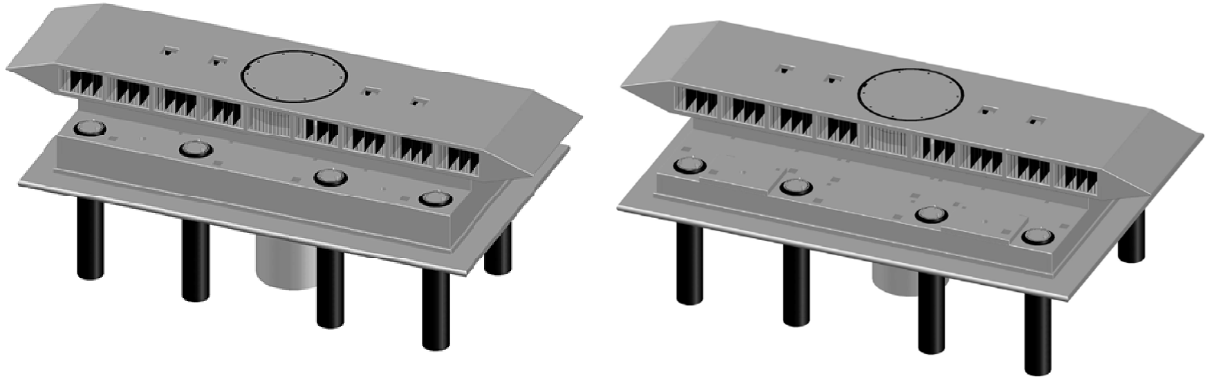
Figure 5: 3 Dimensional views of the intake heads (Type 1 on the left and Type 2 on the right; only the foundations are different; hydraulic performance are the same for both types)
