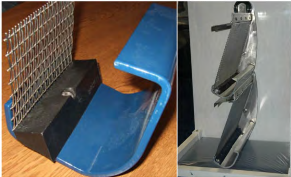
Figure 17: Basic band screen bucket in profile
