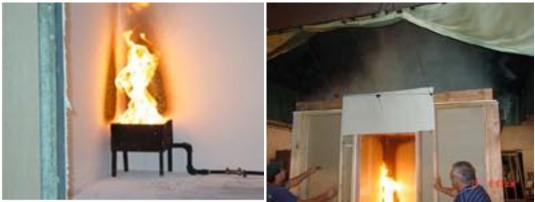
3. NFPA 286 has a specific definition of flashover, but specifies no acceptance criteria. Acceptance criteria are specified in Section 803.2.1 of the NCBC, one of which is the room must not flashover during the 160 kW exposures.
