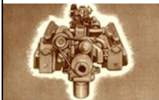
Caption: "Rear Engine - 166 horsepower, flat opposed six-cylinder engine located below the level of passengers. Aluminum alloy construction. More power for the weight of the car than any volume production automotive engine ever built. Eliminates fumes, heat, noise in passenger compartment."
