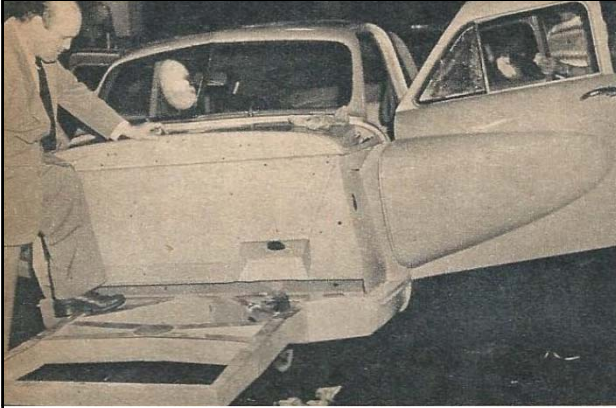
Above: caption: "Where's the engine? It's not up front, Tom discovered. It's in the rear, leaving the front free for lots of baggage." 583
