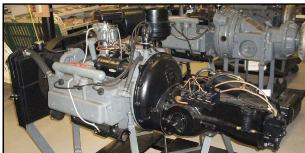
It was also becoming clear that many of the breakthrough designs Tucker called for and featured in their early advertisements could not be implemented (at least not at the car's projected selling price of $2,450). The Ben Parsons designed flat-six (589 cu. in.) engine was proving troublesome, so the decision was made to fit production models with a Franklin six-cylinder engine. As well, an Alex Tremulis design for a fastback sedan body style (with conventional seating for six) was chosen for the final design.
