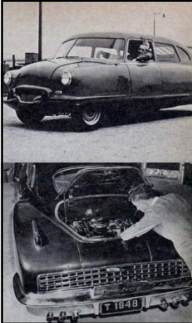
Left T&B: caption: "Man with flying hair, top, is W.B. Stout, who is testing aft-engine car he built of glass. The fabulous Tucker, bottom, gets its push from the 150-hp motor in the rear. Note the six exhausts."
