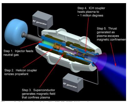
Figure 2. Schematic of the VASIMR VX-200 engine.
