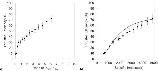
Figure 4. Thruster efficiency of the VX-200 engine as a function of the ICH RF Power to Helicon RF Power, left, and as a function of specific impulse, right. A least squares fit of the data to a semi-empirical model is also superimposed, right.
