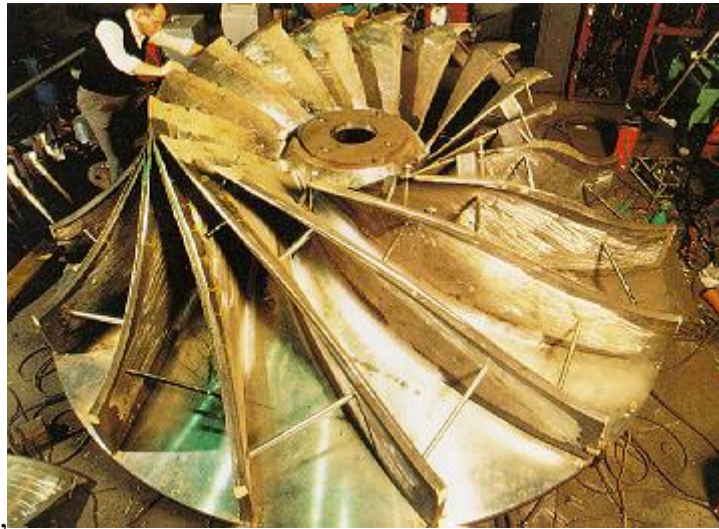
Fig. 4.5. Fabrication of a runner with splitter blades in the workshop at Kvaerner Energy A.S. Note: Only the full length blades are welded in the picture of the runner. (See also fig. 10.7 chapter 10 where all the splitter blades are also welded to the crown of the runner.)
