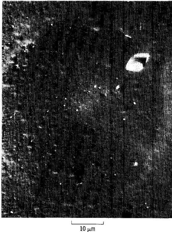
FIGURE 19-9.—Mica surface from the shaded portion of the LSCRE. Etching and microphotography conditions were the same as those for figure 19-5.
