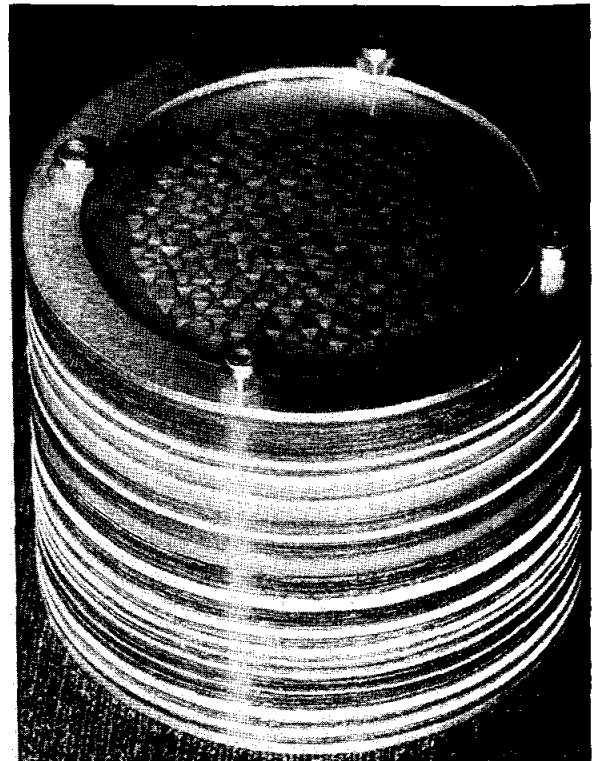
FIGURE 25-1.—Biostack software composed of biologic layers and sheets of radiation detectors.
