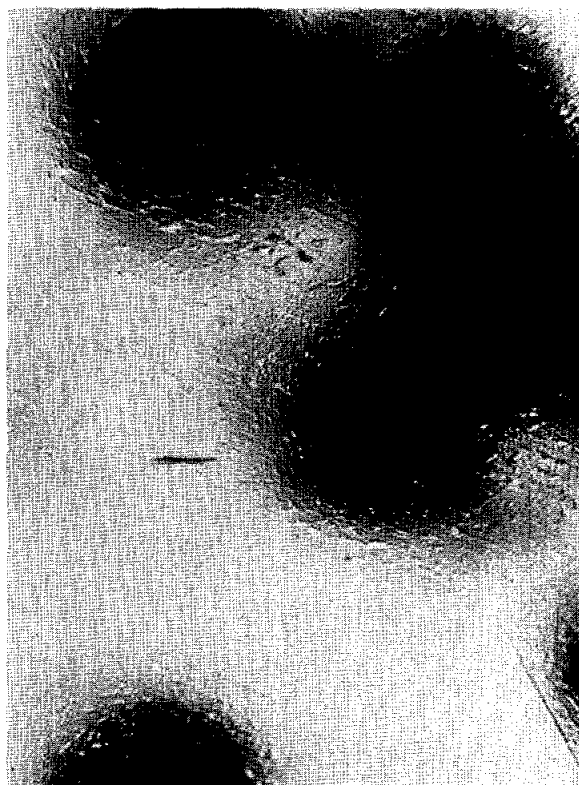
FIGURE 25-11.—Eggs of Artemia salina on a CN sheet of the biostack II flight unit and the track of a hitting HZE particle.
