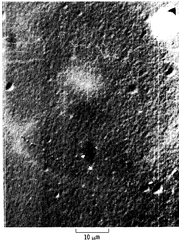
FIGURE 19-8.—Mica surface from the sunlit portion that was covered with 150 nm of silver during exposure. Etching and microphotography conditions were the same as those for figure 19-5.
