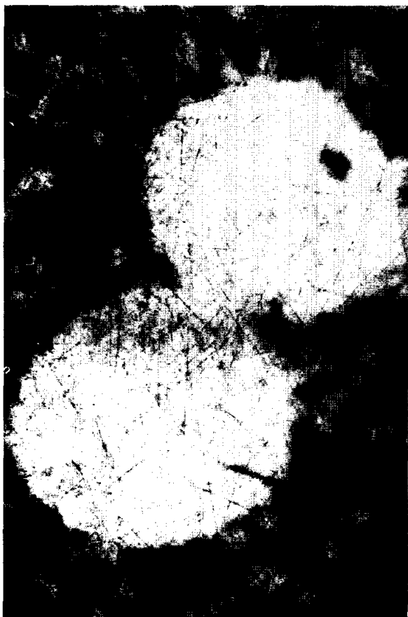
FIGURE 25-10.—Shadows of two Artemia salina eggs on the K2 emulsion of the biostack II flight unit and the track of an HZE particle hitting an egg.
