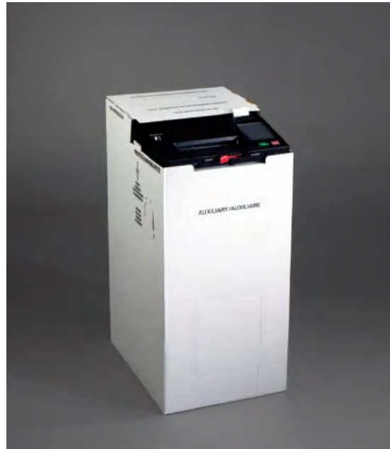
The ImageCast Precinct tabulator on top of the large cardboard ballot box
