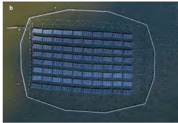
FIGURE 2.9. Solaris Synergy design: Floats (a), outer ring (b) and an illustration of automatic wind adaptation (c).
