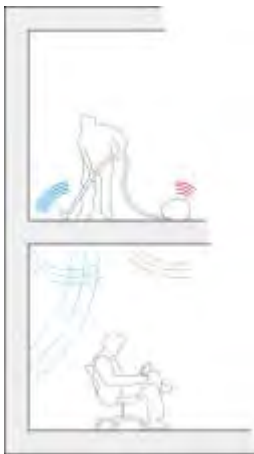
Figure 13: Excitation by airborne sound in the emission room and emission of airborne sound in the reception room
