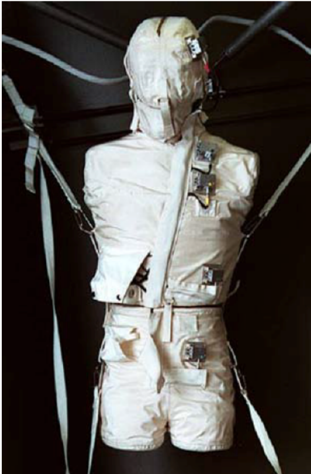
Figure 3.1: NASA uses an anatomical model of a human torso and head that contains more than 300 radiation sensors.
