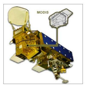
The Moderate Resolution Imaging Spectroradiometer (MODIS) instrument is designed to provide observations that scientists can use to increase understanding of global dynamics and processes occurring on the surface of the Earth and in the lower atmosphere.
