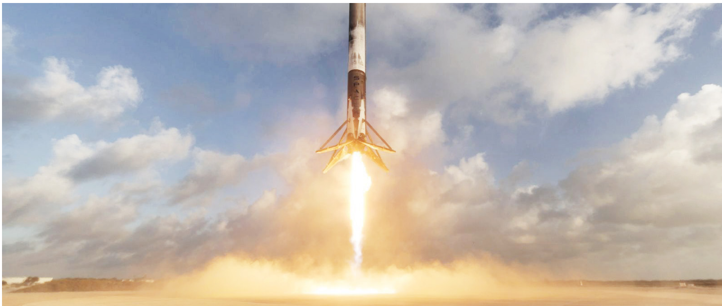
Fig.2. Falcon 9 completing a successful propulsive landing
