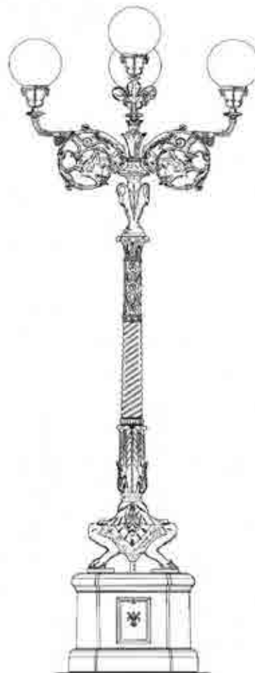
Candelabro modello MI L5 ZL H mm 4060 KG 496 - AEC
