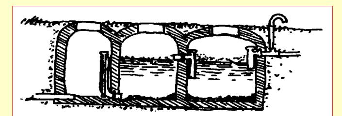
The first septic tanks appeared in the United States about 1883, when a two-chamber, round, vertical tank equipped with a dosing siphon for discharge was designed by Edward S. Philbrick of Boston, Mass.
