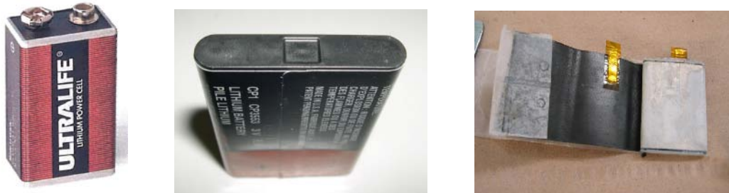
Figure 8: Prismatic Li cell constructions
