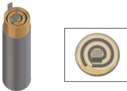
Figure 40: LSX 14500 cell construction and coiled Li/C electrodes
