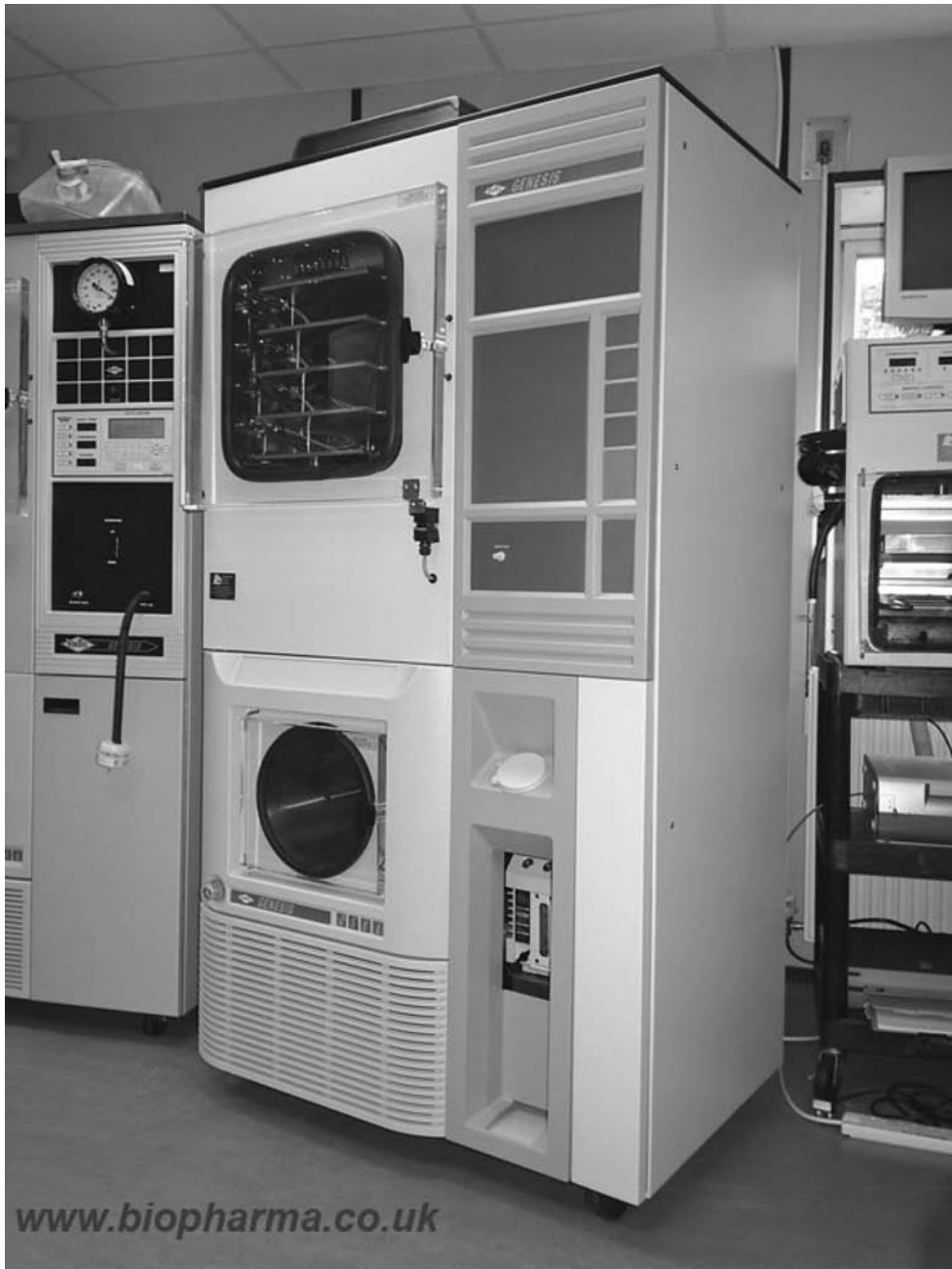
Fig. 12.5 Larger laboratory shelf-style freeze dryer. The shelves are temperature controlled and are located in the upper part of the equipment behind the glass window. The condenser lies in the lower half (behind the black circle). Reproduced with kind permission from Biopharma Process Systems Ltd. ( www.biopharma.co.uk ).
