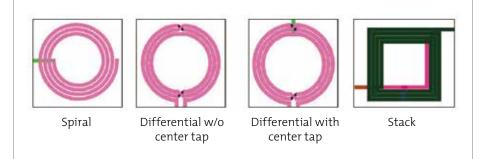
The GUI based VIL can be used to simulate all types of RF inductors.
