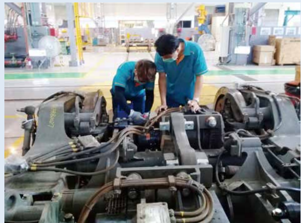
轉向架馬達墊片檢查 Inspect bogie gasket
