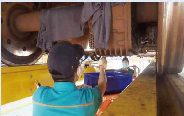
聯軸器換油 Change oil on coupling
