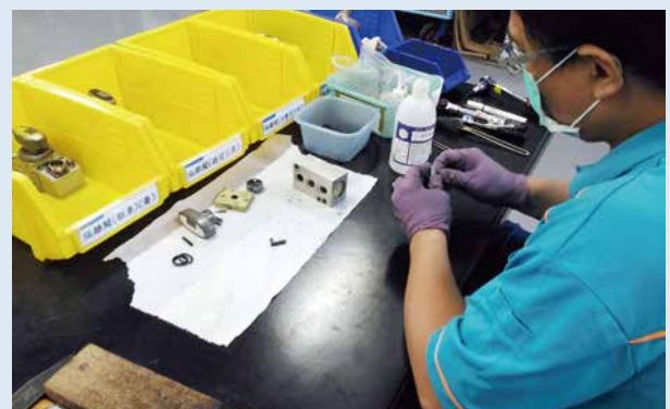
煞車控制模組氣壓閥件檢修 Repair pressure valve of break control module
