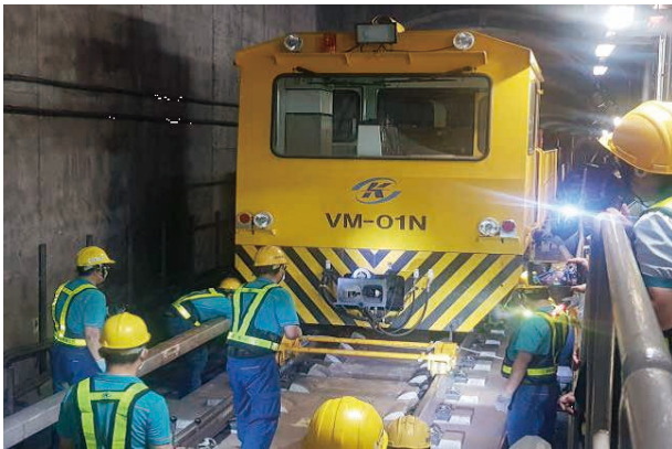
搶修人員安裝車輪組滑行者 Repair crew installing a wheel set skid
