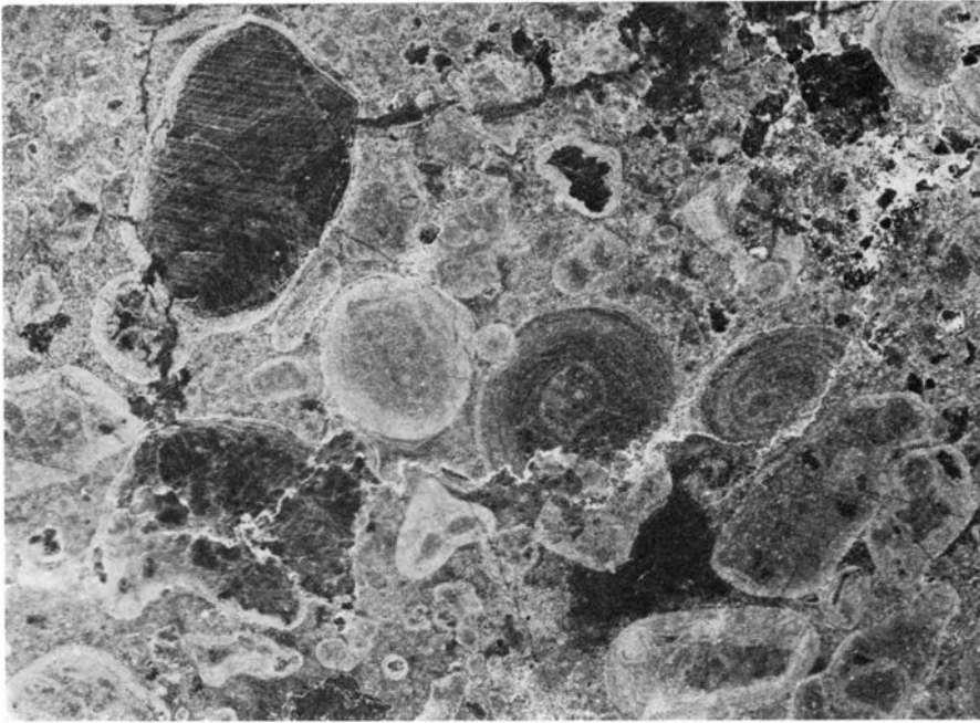
Fig. 9. Peel of ooides from the Biri Formation. The ooides in the centre of the picture are partly dissolved by stylolites. Heggeli, Biri district (61.20–82.30). Width of section 1 cm.
