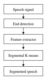
Fig. 1. Block diagram of the phoneme segmentation procedure
