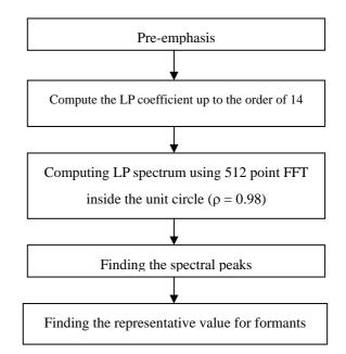
Fig. 4. Block diagram of formants extraction procedure
