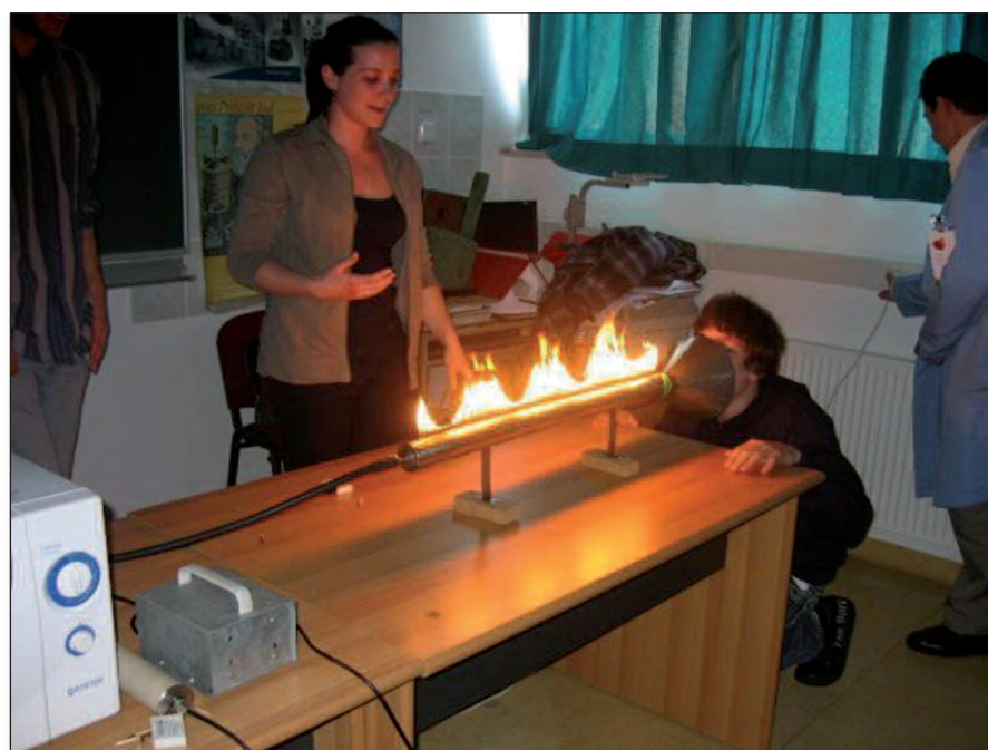
▼ FIG. 3: Physics Express visiting an elementary school in Rijeka. Ines Filipas from Physics Express explaining the exercise entitled "Rubens tube", while one of the students is trying to induce the tube standing waves by identifying the right frequency with his voice.
