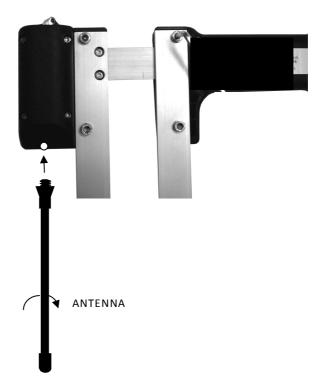
Data can be sent online when the user presses Enter, see **Line**. Data can also be sent as a file, including all stored registration, see **PC**. Make sure to set the caliper in Radio mode when using the Radio. Choose **Rdio** instead of **IR** in the **SET menu**. The receiver can be used in any PC compatible 9 pin serial port.
