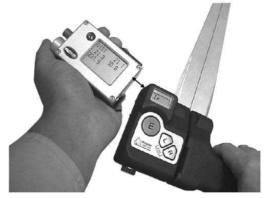
The IR reading can be stopped by pressing ESC on the Digitech caliper (L + R buttons).
