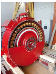
Traction motor generation on permanent magnets system 400 kW, 130 rpm
