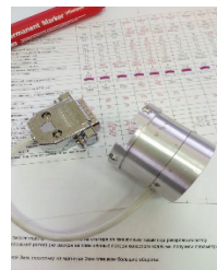
Synchronous micromotor for drive of cryogenic 25 W, 4000 rpm
