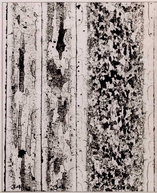
Fig.4 Two pieces of 34 gauge sheet and one piece of 28 gauge sheet, water quenched after 10 minutes in nitrate bath at 510°C. Mag.100X, Etched HF-HCl. 7557 A.S.
