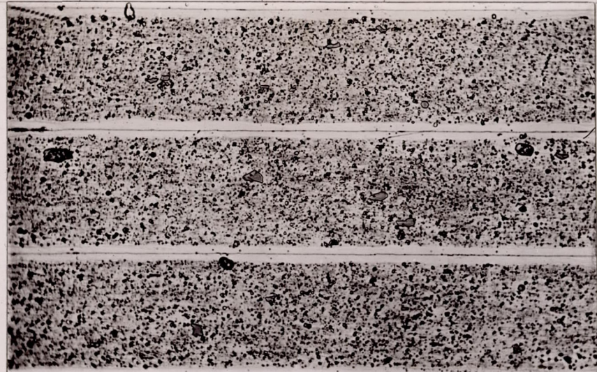
Fig.7 Full cross section of three pieces of 17SH foil 0.0017" thick rolled from the sheet shown in Fig.6 before heat treatment. Mag.500X, Etched 1/2% HF.
