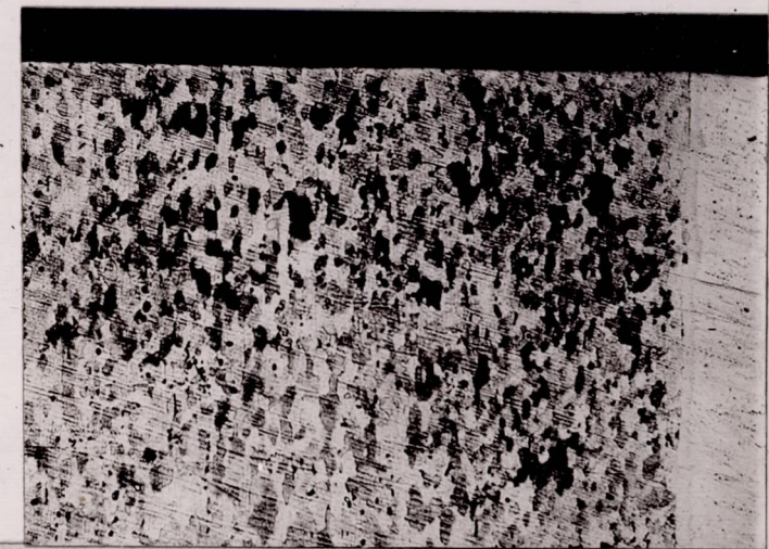
Fig.9 Illustrates a similar edge of 14 gauge "Alclad" 17ST sheet exposed during the same period as the normal 17ST. Mag.100X, Etched 1/2% HF.
