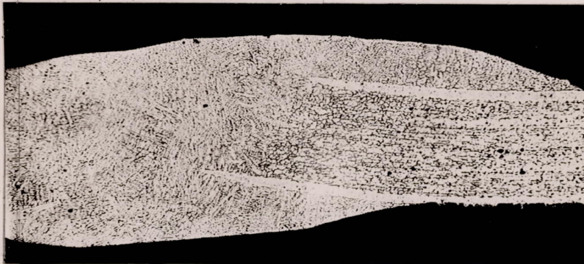
Fig.10 Shows intergranular attack along the edge of 7/16" 20 guage 17ST channel after 48 hours alternate immersion in salt-hydrogen peroxide solution. Mag. 100X, Etched 1/2 % HF.
