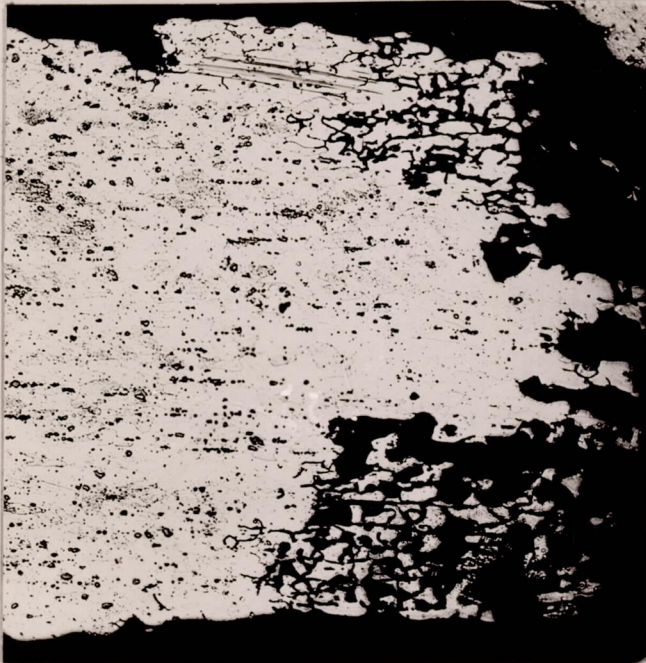
Fig.10 Shows intergranular attack along the edge of 7/16" 20 guage 17ST channel after 48 hours alternate immersion in salt-hydrogen peroxide solution. Mag. 100X, Etched 1/2 % HF.
