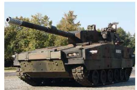
EOTS mounted on a Obrum light tank (Demonstrator)
