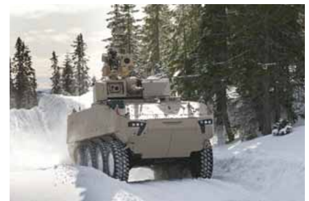
EOTS mounted on a Piranha armoured fighting vehicle
