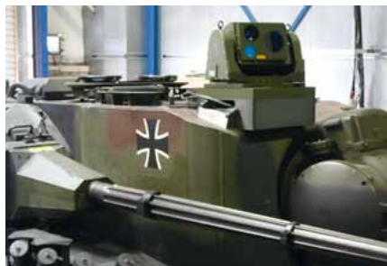
EOTS mounted on a Gepard anti-aircraft tank
