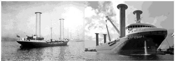
Figure 1: One of the first rotor ships, the *Buckau* (left), and the present-day rotor ship *E-Ship 1* (right) Source: wikipedia.org (accessed on 10 August 2012, right photo by Carschten)
