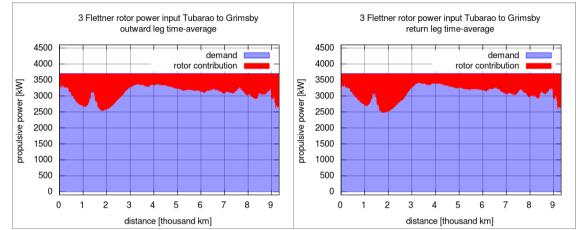
Figure 3: Time-averaged propulsive power generated by a set of three Flettner rotors, plotted as a share of the main engine power requirement of a slow-steaming, 50,000 dwt bulk carrier (cf. section 2.1 and 2.2). Left: On the way from Tubarao to Grimsby. Right: Returning from Grimsby to Tubarao. Data: Authors
