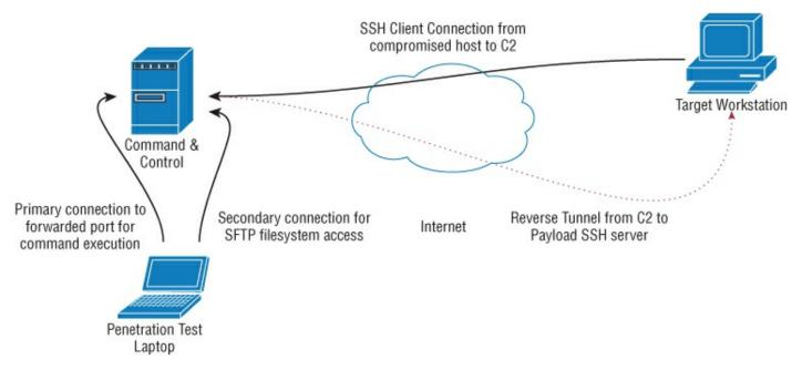
**Figure 1.11:** Initial basic Command and Control infrastructure.
