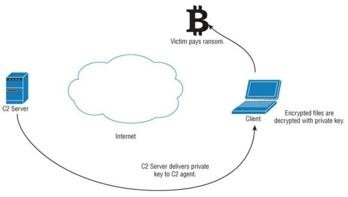
Figure 5.4: Decryption process flow.
