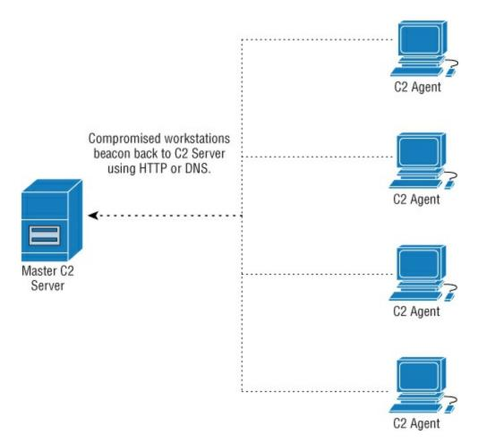
**Figure 8.1:** Initial beacon designated as Master node.
