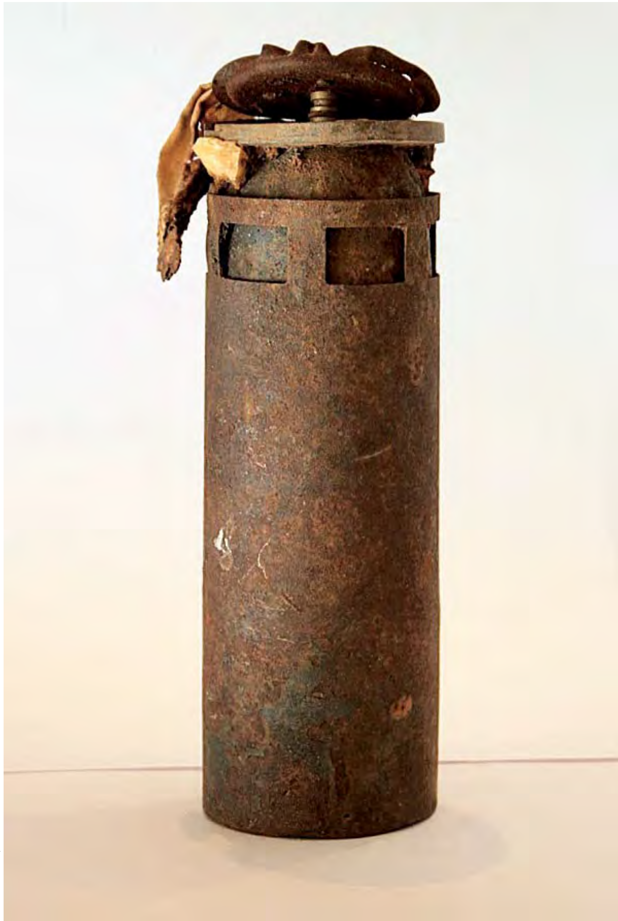
Figure 25: BLU-97 submunition, damaged by frequent burning of the grass
