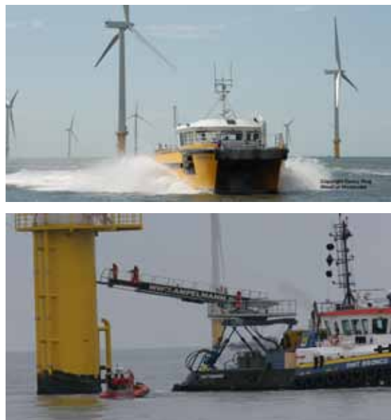
FIGURE 31: Two new access systems, Windcat Workboat (top) and Ampelmann (below)
