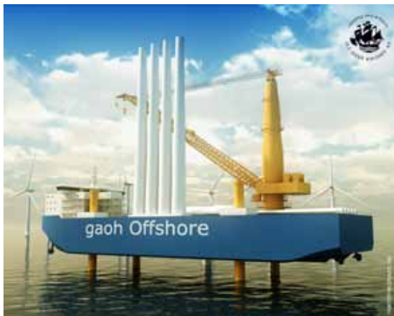
FIGURE 32: Example of the Gaoh concept. This boat is designed to lift 18 3.6 MW turbines in 45m depth, including seabed penetration
