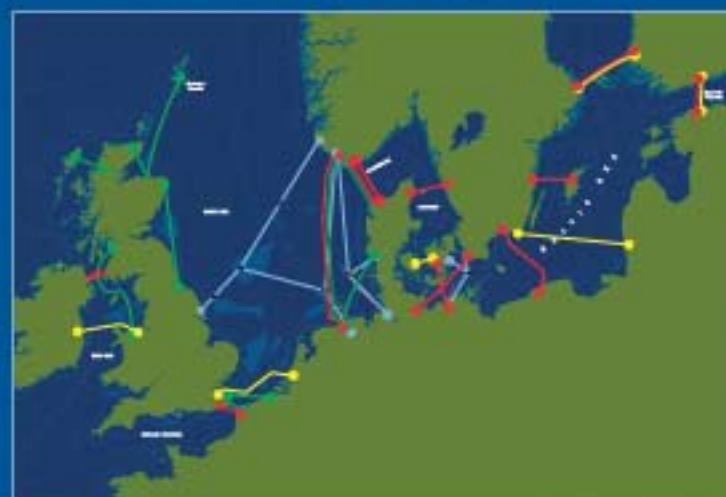
FIGURE 14: Offshore transmission lines in 2020 based on current TSO plans and studies, amended by EWEA as appropriate
