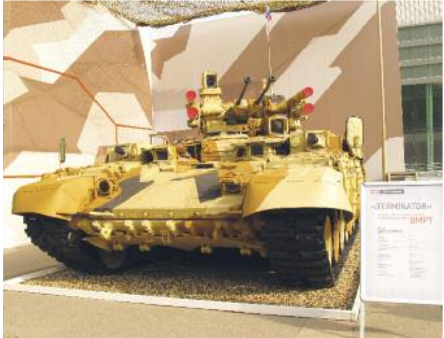
Based on a tank chassis, the Terminator is a support vehicle featuring an impressive firepower, developed by Uralvagonzavod (Armada/P. Valpolini)
