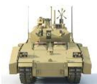
A series of views of BAE Systems GCV study: the company decided to adopt a hybrid electric drive propulsion based on its Traction Drive System and QinetiQ E-X-Drive transmission. (BAE Systems)
