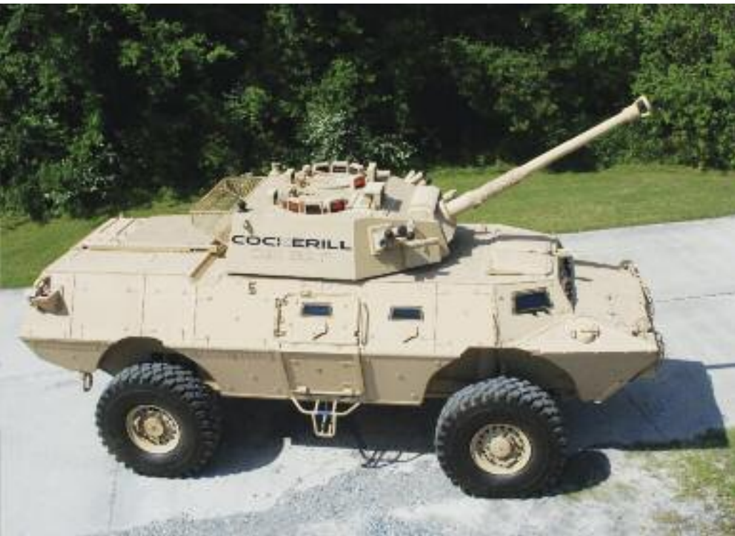
The Select variant of the Commando family is the base for the Afghan National Army Mobile Strike Force Vehicle, part of which are equipped with the CMI 90 turret. (Textron)
