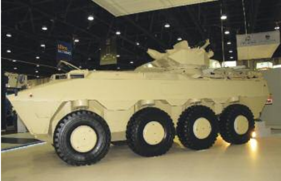
An FNSS PARS 8x8 sporting the company's one-man Sharpshooter turret; a derivative of this infantry fighting vehicle has been sold to Malaysia equipped with a Denel 30 turret that is still being developed. (Armada/P. Valpolini)
