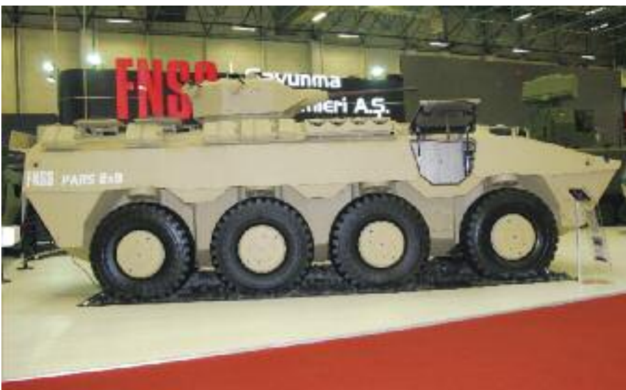
The PARS 8x8 features semi-automatic computer controlled pneumatic suspensions that allow to compensate lateral inclination. (Armada/P. Valpolini)
