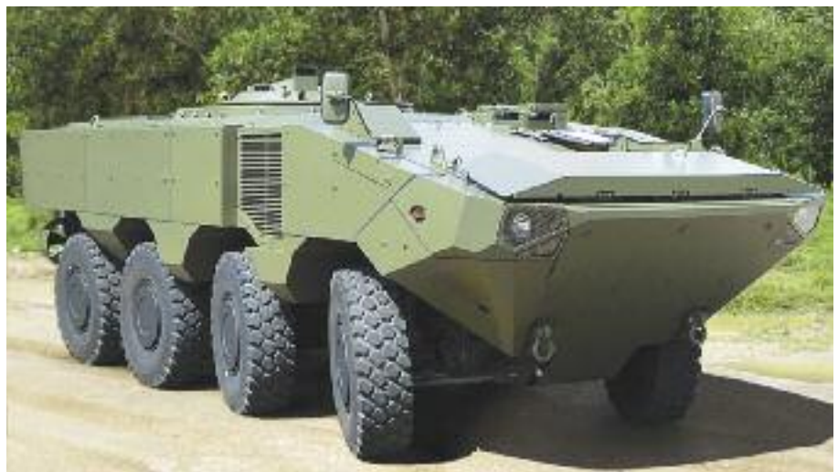
BAE Systems teamed with Iveco DV for answering the US Marine Corps requirement for the Marine Personnel Carrier; the vehicle is a derivative of Iveco's SuperAV. (BAE Systems)
