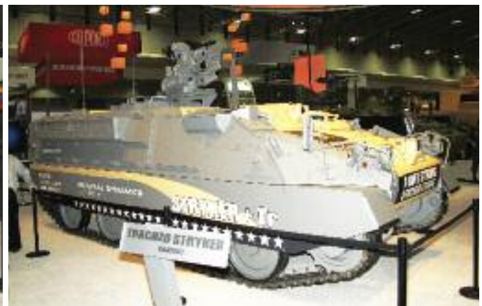
One of GDLS answers to the AMTV programme is the Stryker +Tr, a tracked version of the Stryker unveiled in 2012, with a weight of 30 tonnes and an 8-tonne growth potential. (Armada/P. Valpolini)
