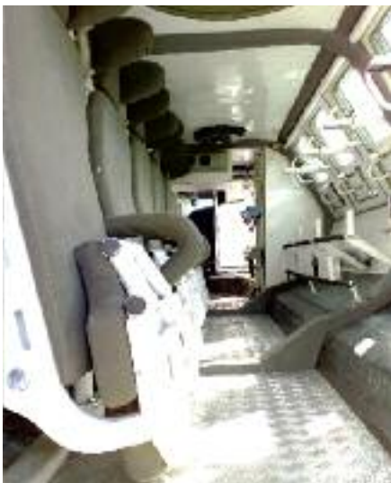
The inside of the Lazar 2 troops compartment; soldiers have a direct view of the surrounding scenario and can use their individual weapons from inside the vehicle. (Yugoimport)
