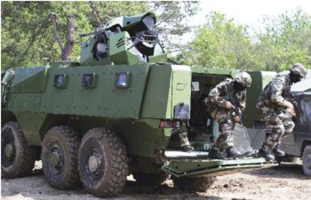
The latest version of the VAB is the MkIII, that can host 10 dismounts plus crew in a 13 m 3 volume protected up to Level 4 ballistic and 3b antimine. (RTD)
