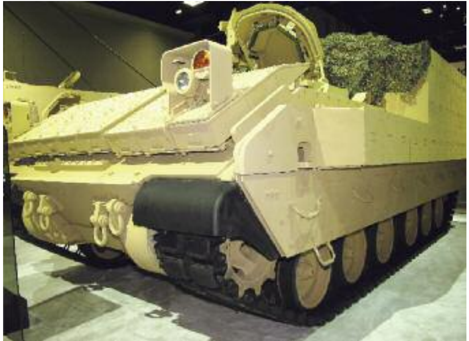
For the AMPV programme BAE Systems offers a vehicle based on the Bradley chassis, many of which are available in Army depots. (Armada/P. Valpolini)
