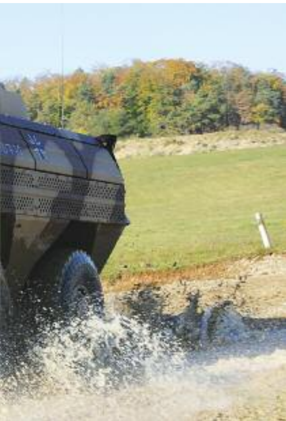
The latest version of the VAB is the MkIII, that can host 10 dismounts plus crew in a 13 m 3 volume protected up to Level 4 ballistic and 3b antimine. (RTD)
