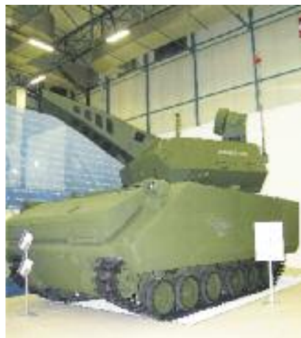
The ACV30 was developed by FNSS to answer the Turkish Army requirement for an amphibious air defence artillery system. Weighing in at 30 tonnes, the vehicle is necessarily huge to allow proper flotation. (Armada/P. Valpolini)
