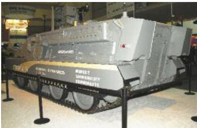
One of GDLS answers to the AMTV programme is the Stryker +Tr, a tracked version of the Stryker unveiled in 2012, with a weight of 30 tonnes and an 8-tonne growth potential. (Armada/P. Valpolini)
