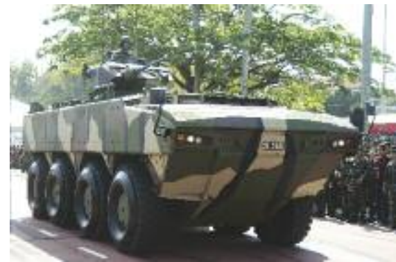
The AV-8 is the Malaysian 8x8 vehicle being built by DefTech, that is heavily based upon the FNSS PARS 8x8 armoured infantry fighting vehicle. (FNSS)
