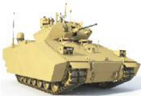
A series of views of BAE Systems GCV study: the company decided to adopt a hybrid electric drive propulsion based on its Traction Drive System and QinetiQ E-X-Drive transmission. (BAE Systems)
