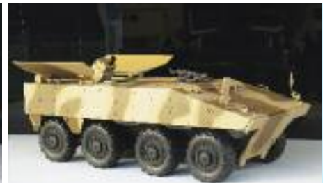
Nexter plans to add numerous versions of its VBCI to the current AIFV and command post versions: from left to right these scaled models of the recovery, AIFV with Eastern Europe ordnance, and the mortar carrier versions. (Armada/P. Valpolini)
