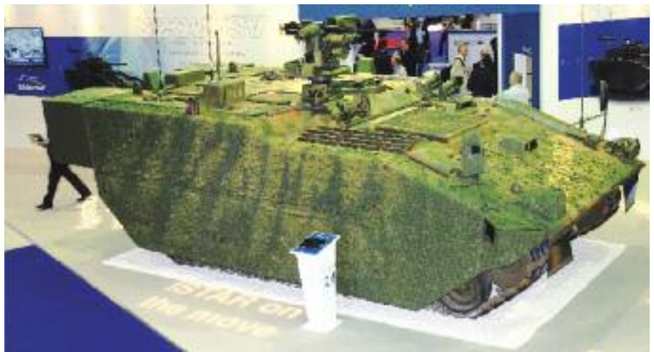
General Dynamics UK Specialist Vehicle Mobile Test Rig was exhibited at DSEI 2013 in the Protected Mobility Reconnaissance Support configuration, fitted with a Kongsberg Protector armed with a 12.7 mm machine gun. (Armada/P. Valpolini)
