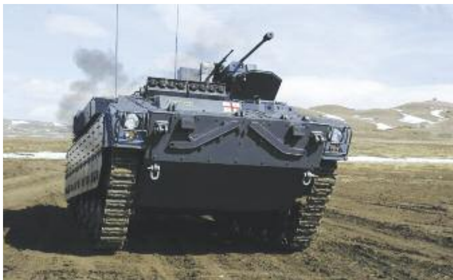
South Georgia is one of the latest countries to enter the armoured vehicles production arena; the Lazika 14 tonnes APC can carry up to seven dismounts and three crew members. (Internet)
