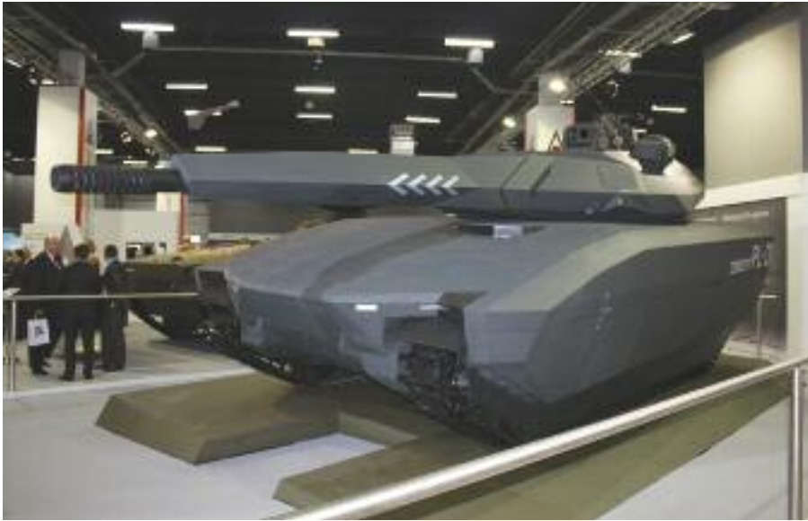
At MSPO 2013 in Poland BAE Systems and Polish Defence Holding unveiled the PL-O1 concept support vehicle based on the Universal Tracked Platform. (BAE Systems/PDH)
