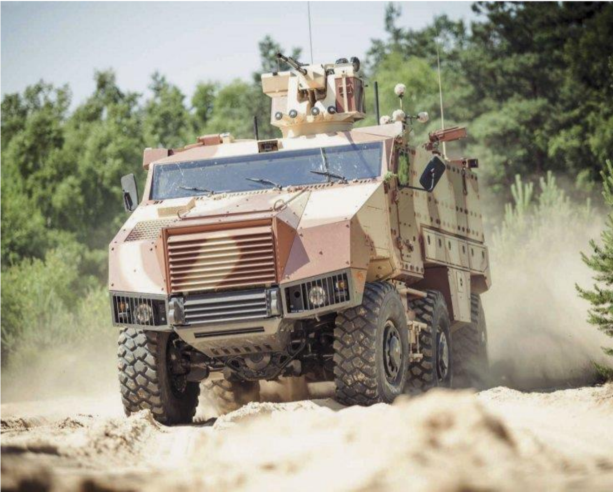
The Nexter Systems TITUS 6x6, developed for the export market, is based on a Tatra chassis to provide a high level of cross-country mobility. It is shown here fitted with the Nexter Systems ARX20 RWS armed with a 20 mm cannon and 7.62 mm MG. (Nexter Systems)
