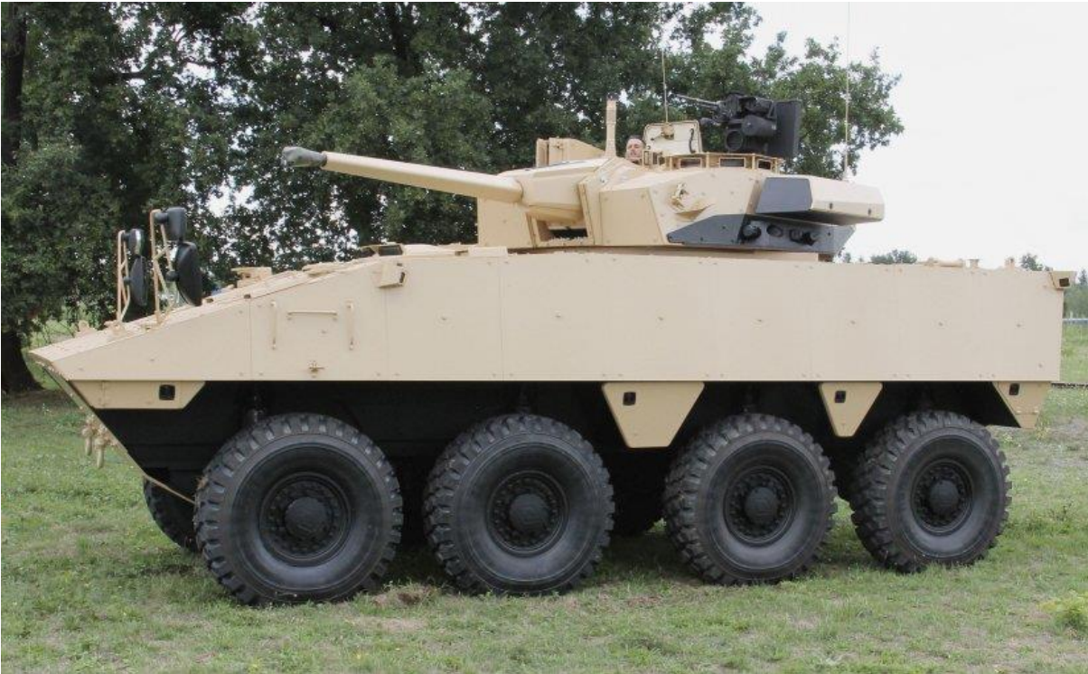
The latest Nexter Systems VBCI-2 8x8 infantry fighting vehicles feature a new Nexter Systems two-person turret armed with the 40 mm Case Telescoped Armament System. (Christopher F Foss)
