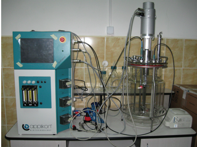
Fig. 5. General view of the Laboratory scale bioreactor (15 L)
