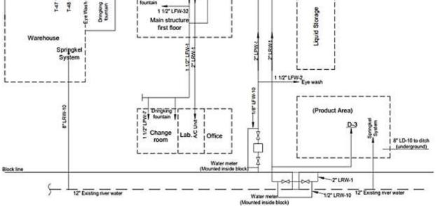
Figure 6: Standard type layout for service piping diagram
