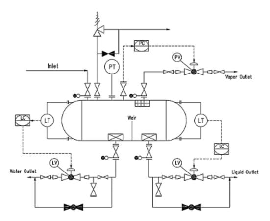
Figure 4: Typical P&ID arrangement for 3 phase separator vessels
