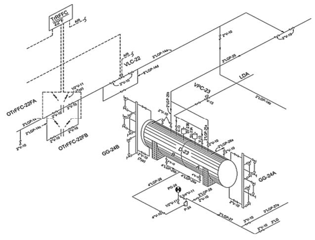
Figure 5: Piping details isometric diagram
