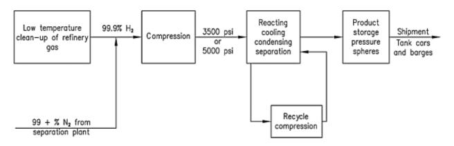
Figure 1: Block flow diagram of Ammonia Process
