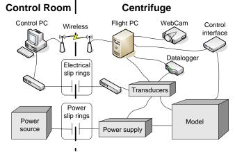
Figure 4 Centrifuge control and data acquisition system
