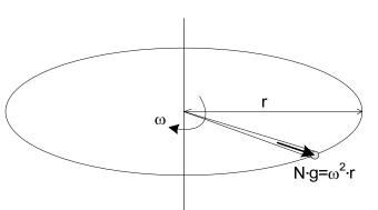
Figure 1 Acceleration by rotation
