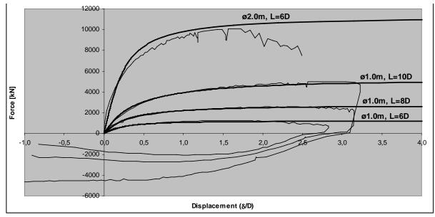
Figure 10 Load-displacement curves for pile tests.
