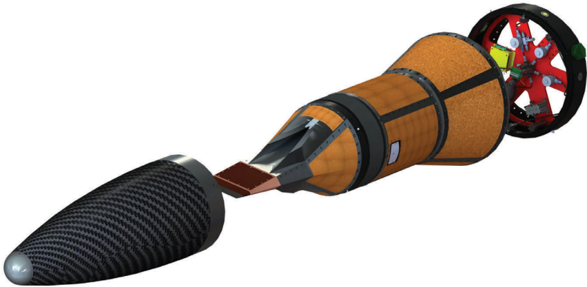
Figure 3.3 Australian–U.S. HIFiRE Scramjet
