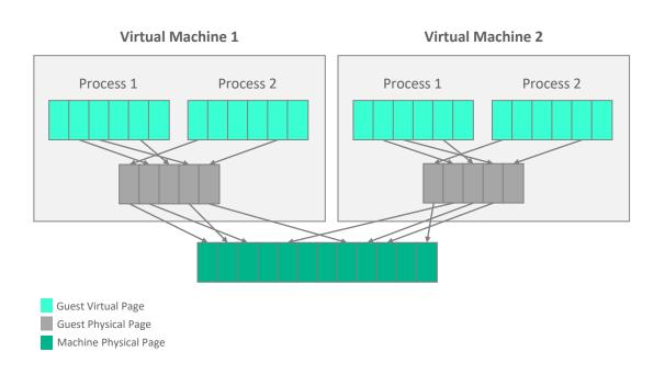
typedef struct ept pte { uint64 read : 1; // bits 2..0 : 1; // bits 2..0 uint64 write : 1; // bits 2..0 uint64 execute : 3; // bits 5..3 uint64 ept mt :1; // bit 6 uint64 ignore pat mt uint64 is large page :1; // bit 7 uint64 accessed :1; // bit 8 :1; // bit 9 uint64 dirty :1; // bit 10 uint64 user execute uint64 ignored1 :1; // bit 11 uint64 pfn : 40; // bits 51..12 : 11; // bits 62..52 uint64 ignored2 uint64 supress ve :1; // bit 6
