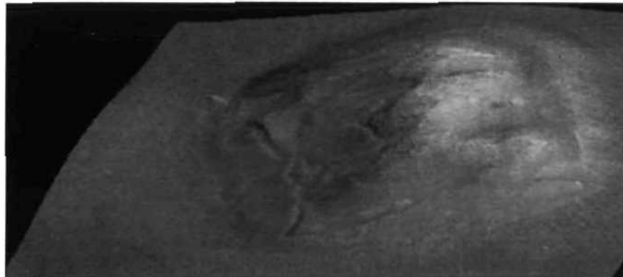
3-D perspective view of the Face on Mars landform produced from the April 8, 2001, Mars Orbital Camera image and all the available laser altimeter elevation measurements by Mars Global Surveyor's MOLA laser altimeter.
