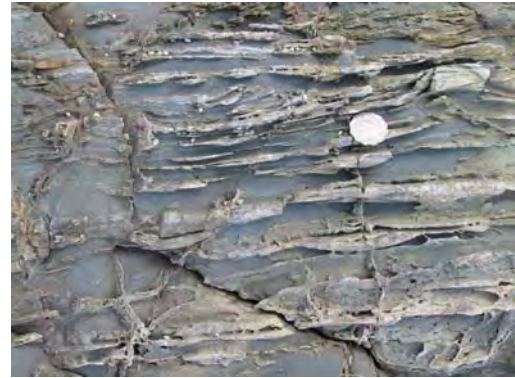
Differential weathering in the interbedded siltstone and sandstone – laminae or lenses of quartz sandstone are more resistance to weathering than the siltstone, so they protrude above the weathered rock surface
