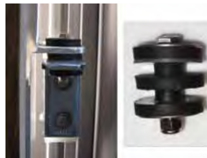
Fig. 8. Bolt assembly through tab and bracket showing Sorbothane® with stainless steel washers surrounding top, middle, and bottom pads (Photo: Gerri Strickler © 2012 Museum of Fine Arts, Boston).
