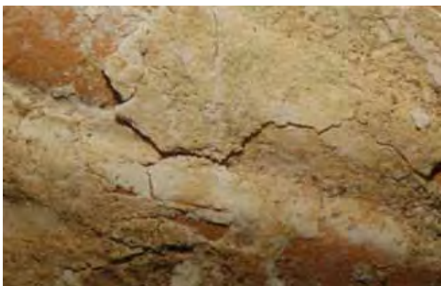
Fig. 4. Degradation of white kaolin layer (photomicrograph x25) (Photo: P. Bonev).
