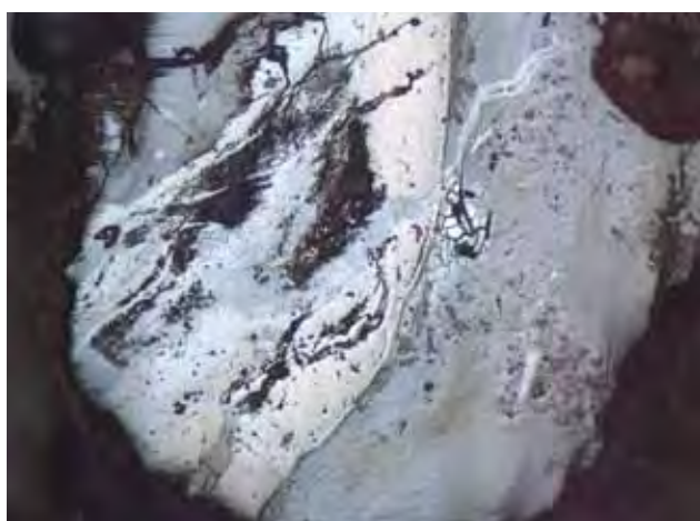
Fig. 6. Microphotograph (magnification 200X) of highly corroded forged iron from AK-MAK-66-A (Photo: Arie Wallert, Rijksmuseum, Amsterdam).
