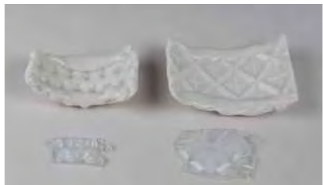
Fig. 3. B-72 castings and moulds from pressed and cut glass (Photo: The Corning Museum of Glass).
