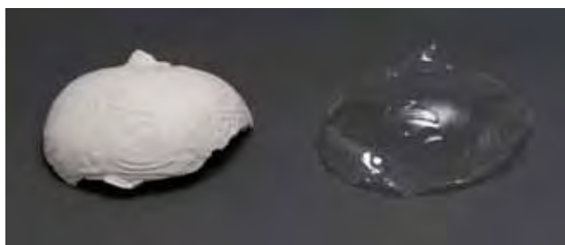
Fig. 7. Plaster form (Height: 7.1 cm, Width: 9.8 cm, Depth: 4.5 cm) next to formed PVC mould wall showing good conformity (Photo: The Sherman Fairchild Center for Objects Conservation, The Metropolitan Museum of Art. Image © The Metropolitan Museum of Art).
