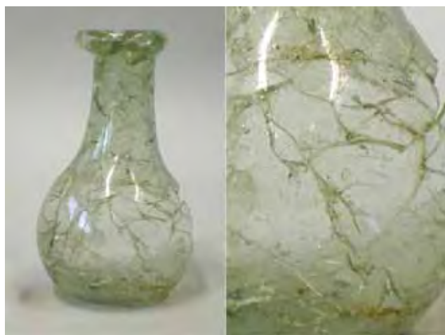
Fig. 2. Glass bottle with internal fractures; the overview (left) and the close-up (right) shows the characteristic crack pattern; strong fragmentation/sugaring, especially at the spout (HA 132_146-9, dated 4th century A.D. (Photo: LVR-LandesMuseum Bonn).
