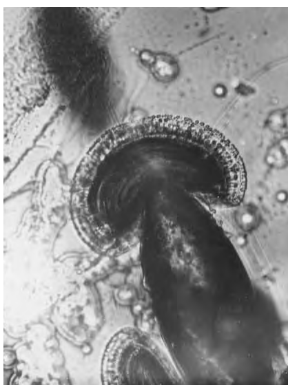
Fig. 9. Banded spot with a corona developed on the tip of an elongated bubble, magn. x200 (Photo: 110a, Geilmann 1955a)
