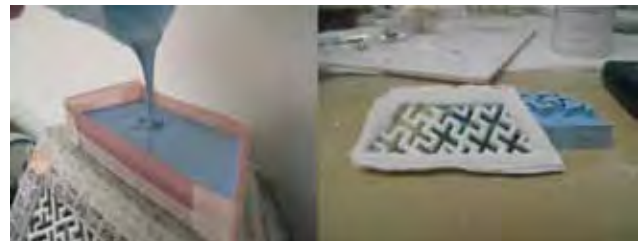
Fig. 3. Open mould with MM903    , a very flexible silicone (Photo: S. Benrubi).
