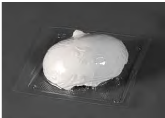
Fig. 5. Plaster form (Height: 7.1 cm, Width: 9.8 cm, Depth: 4.5 cm) with suctioned and cooled PVC foil (Photo: The Sherman Fairchild Center for Objects Conservation, The Metropolitan Museum of Art. Image © The Metropolitan Museum of Art).
