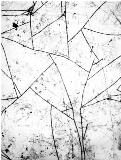
Fig. 6. Sequential development of a crack system – later cracks end at earlier cracks (Photo: 23a, Geilmann 1955a).
