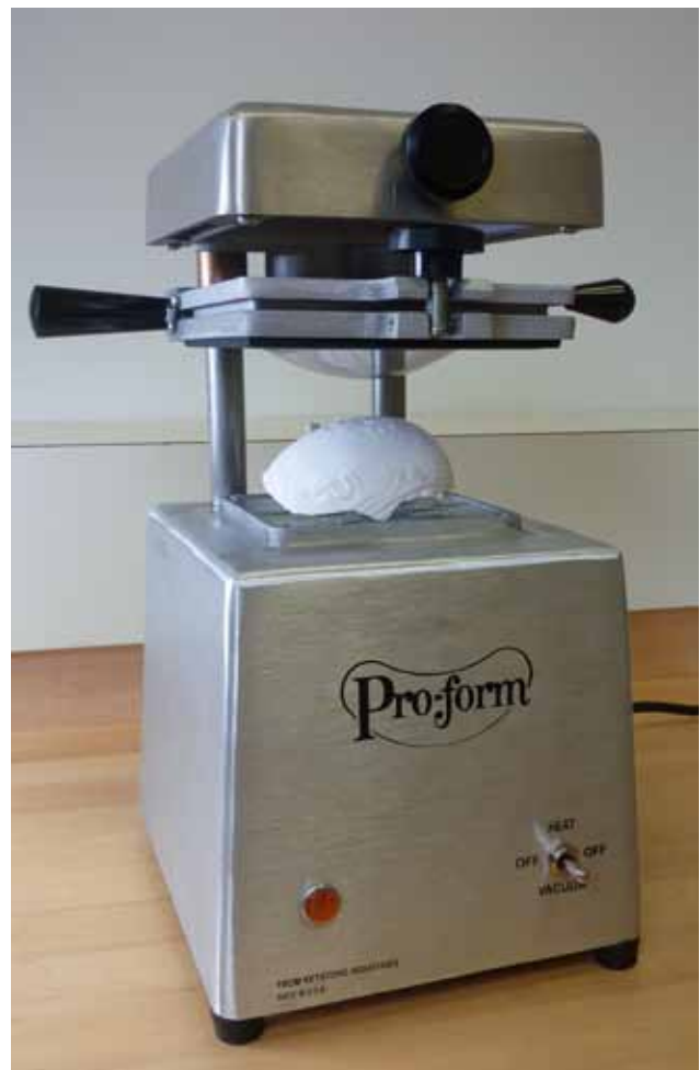
Fig. 4. The Pro-form Dual Chamber Dental Vacuum Former, shown with a plaster form and heated PVC foil in the frame above (Photo: The Sherman Fairchild Center for Objects Conservation, The Metropolitan Museum of Art. Image © The Metropolitan Museum of Art).
