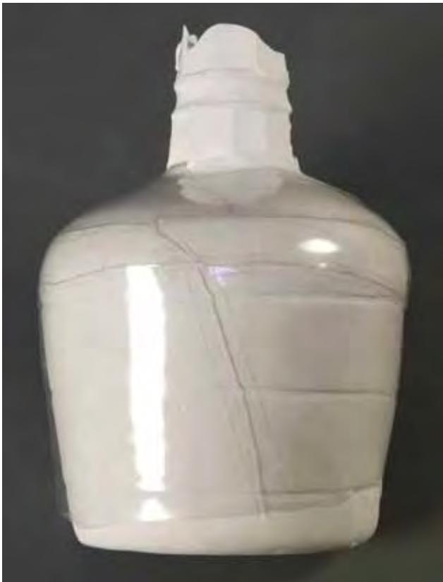
Fig. 3. Pieces of formed PVC cut and pieced together to make a conforming mould wall on a plaster cast (Height: 18.6 cm, Width: 13.1 cm, Depth: 6.5 cm) of a glass vessel (Photo: The Sherman Fairchild Center for Objects Conservation, The Metropolitan Museum of Art. Images © The Metropolitan Museum of Art).
