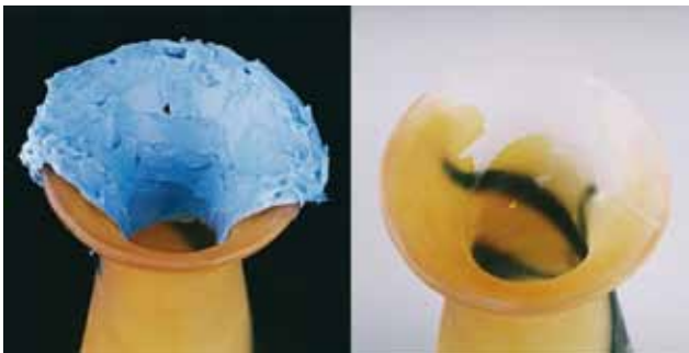
Fig. 1. One-part mould made with the fast-setting silicone Exaflex Regular    (Photo: S. Benrubi).
