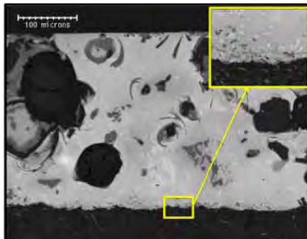
Fig. 9. Backscattered scanning electron microscope image of the cross-section of sample number A152/6/M7 (Schoyestraat, 1590–1613), showing a lot of inclusions in the glaze layer and a sharp transition to the intermediate layer (Photo: M. Vandevijvere).
