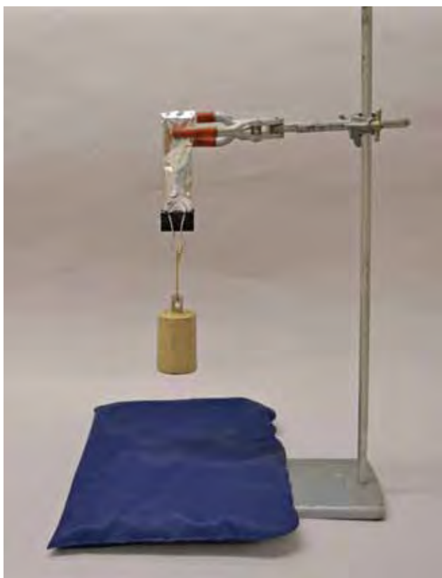
Fig. 4. The bonded sample is suspended from a retort stand with a weight attached (Photo: Hanneke Ramakers © Victoria and Albert Museum, London).
