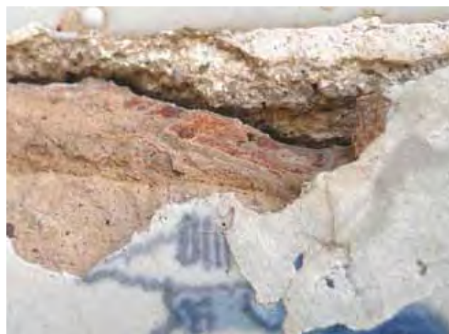
Fig. 5. Salt damage resulting in the delamination of a ceramic body where different clays were mixed in the plastic state. The different clay types (red iron-rich clay and a buff-coloured, calcium-rich clay) are clearly visible (Photo: Kate van Lookeren Campagne).
