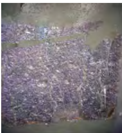
Fig. 1. General view of the top surface of a gold-leaf tessera with greyish alteration. Glass areas with no gold in the middle appear transparent with an aqua hue (stereo-micrograph 20× magnification) (Photo: Polytimi Loukopoulou).
