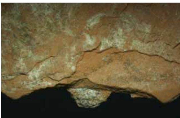
Fig. 6. Characteristic degradation of the ceramic shard, caused by salts (photomicrograph \times 25 ) (Photo: Pl. Bonev).
