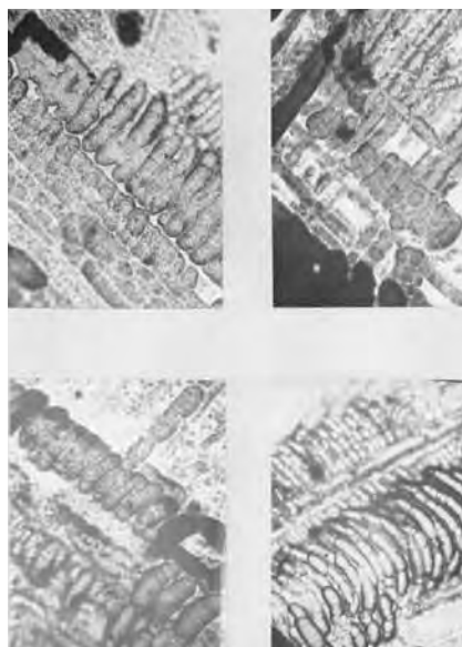
Fig. 3. Photos showing 'chatter marks' heavily etched by corrosion (Photo: page 12, Geilmann 1955a).
