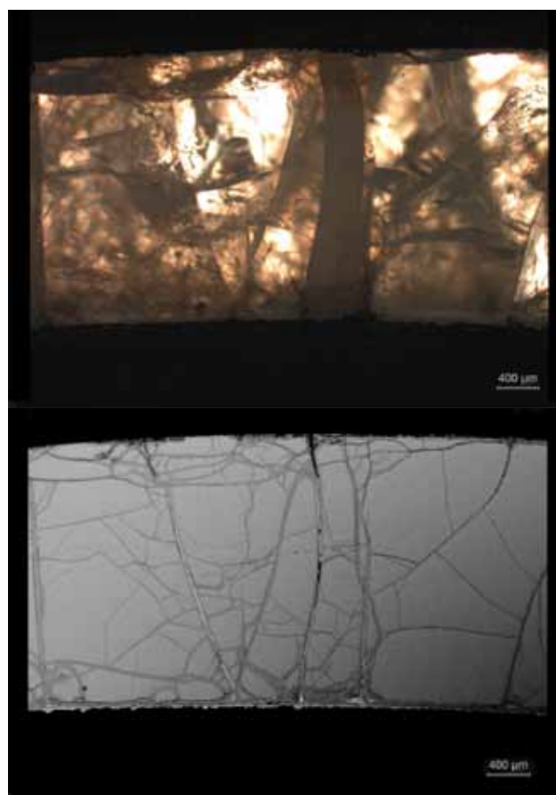
Fig. 3. Cross-section of sugared glass sample (Roman glass, sample H 5699, Martin von Wagner Museum, Würzburg, Germany). Top: light microscopy in transmission light. Bottom: SEM-image (Photo: authors).
