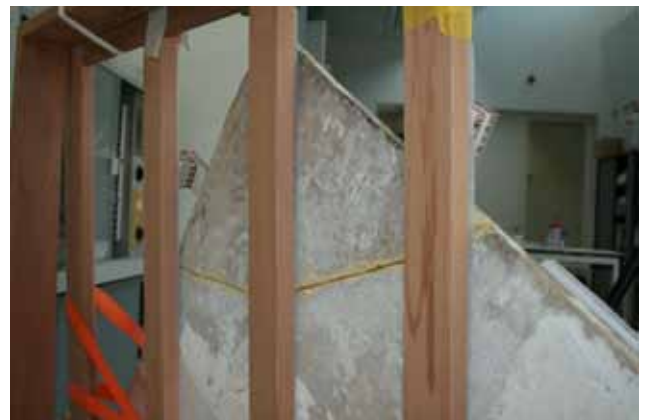
Fig. 1. The first stage of bonding with two pieces vertically secured on the frame in the correct position. When the corner piece was aligned at the front, a crack remained at the back due to the filing-down of the break edges (Photo: author).
