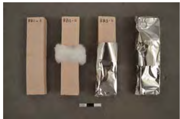
Fig. 3. Sample preparation; the join is wrapped in cotton wool and covered with aluminium foil (Photo: Hanneke Ramakers © Victoria and Albert Museum, London).
