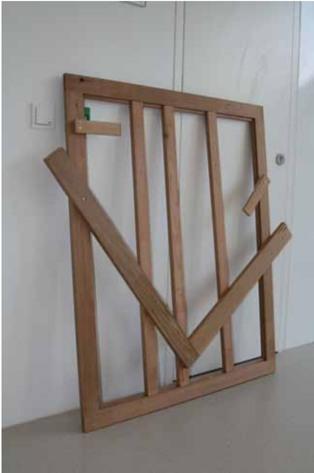
Fig 2. Frame with slats. Wooden strips on these slats held the large piece in the correct vertical position during the first stage of bonding (Photo: author).
