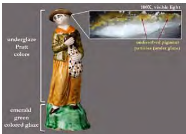
Fig. 2. (left) Sportsman's Companion , c. 1790–1820 (2002.30.15.2) H 18.4 cm W 7.6 cm (Photo: Winterthur Museum), with sample location indicated; (right) cross-section image of underglaze brown.
