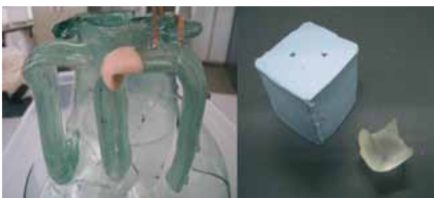
Fig. 2. One-part mould made with the viscous liquid silicone MM903    to cast a detachable fill and the final fill in epoxy resin (Photo: H. Blainpain).
