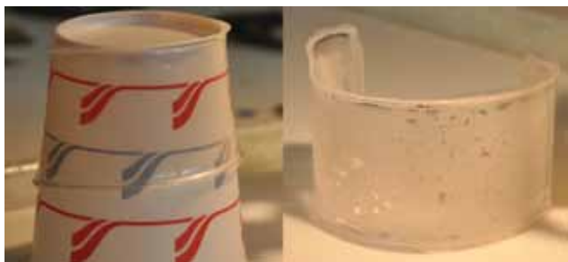
Fig. 4. Making a bubbled film: (a) the B-72 film is placed on a paper cup while still quite flexible and placed in a low temperature oven (40–50°C); (b) the B-72 film with many tiny bubbles (Photo: The Corning Museum of Glass).
