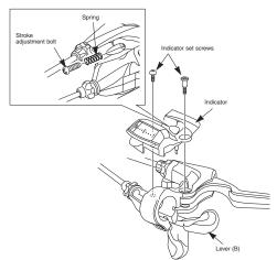
3. Operate lever (B) at least eight times to set the lever to the
