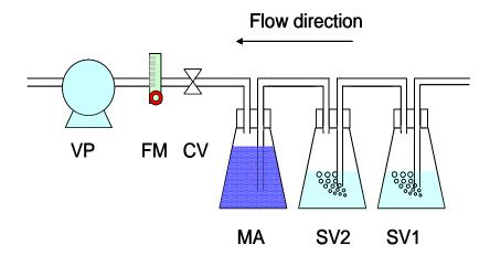
Figure 3-1. Air Sampling System.
