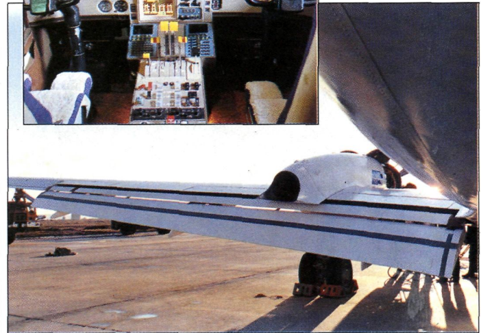
ATP lookalike uses high-lift double-slotted flaps
