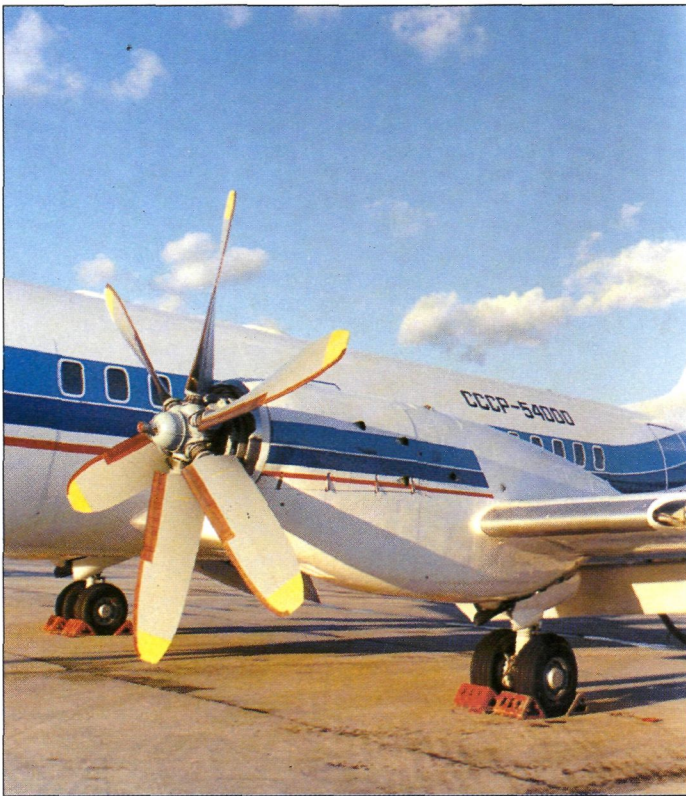
CB-34 propellers use carbonfibre-reinforced composites
