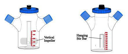
**Note:** Spinning speed needs to be optimized based on the impeller blade used. Start at the lowest spinning speed and incrementally increase the speed until it is optimized to achieve 24–30 hours doubling time, good cell viability, and low cell clumping.
