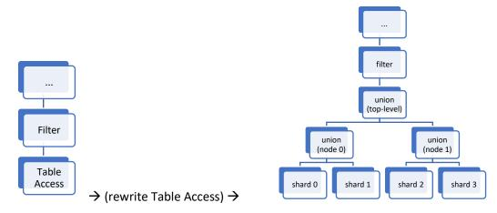
The query optimizer replaces all *Table Access* operators in the RelOp tree with the two-level shard union structure (as illustrated in the diagram). Then the optimizer runs a dedicated distributed optimization pass, relying on the same framework of rewrite rules. These rules attempt to propagate relational operators through the node/shard unions, down to the data shard level, and these are mostly the same transformations as the ones applicable for the regular *Union* operator. In particular:
