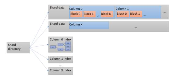
In general, the shard storage format is designed to avoid any non-trivial parsing and minimize the number of I/O operations when accessing the relevant data objects at query time.
