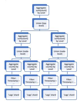
Since the vast majority of queries deal with the uniformly distributed data shards, the query plan above usually has a lot of symmetry. In order to reduce the analysis time, the optimizer always keeps these RelOp trees in a compact, "collapsed" form, where each union has a single source operator, and maintains a separate list of relevant shards or nodes that parameterize the sub-tree. The rewrite rules, in turn, are designed to work with this compact form.
