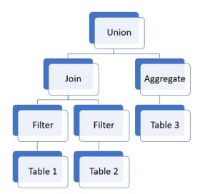
This operator tree is the main representation of the query in the engine; most of the analysis and the optimizations are performed on this RelOp tree.
