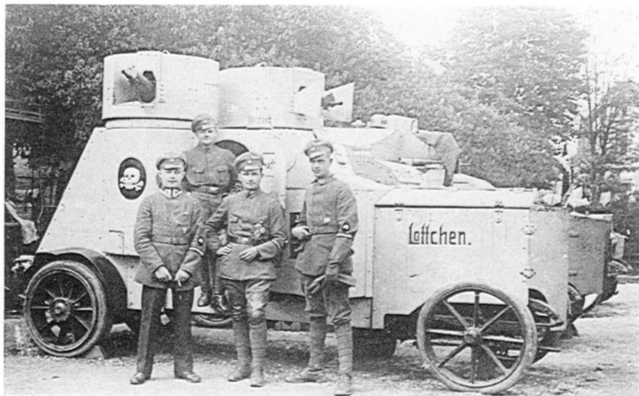
ABOVE: 'Lottchen' was used by a German Freikorps unit in 1919 but had originally been captured in Russia. The make of the chassis is not known but with its twin staggered turrets and 'wings' protecting the water-cooling jackets of the machine-guns the car closely resembles the Izhorskiy-Fiat.
