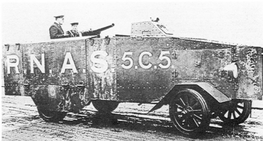
A Seabrook of C Section, Number 5 Squadron, with two of the seven crew manning the 3 pdr. The sides dropped to form a platform for the main armament and four machine-guns. All RNAS armoured car crews were enlisted as Petty Officers.
