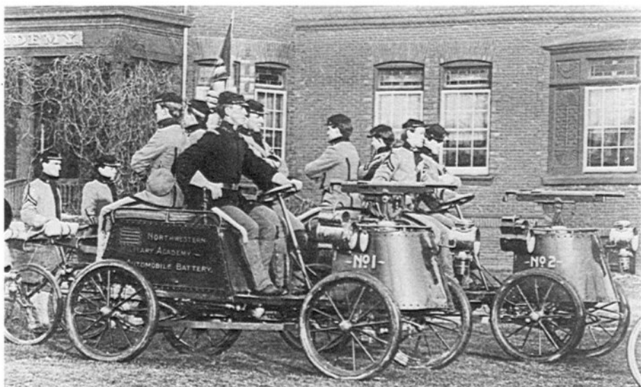
In 1902 Colonel Davidson's students at the Northwestern Military Academy built these two steam cars which were fitted with .30 Colt machine-guns. The cars were unreliable because of the difficulty of maintaining pressure in the boilers, so in 1909 Davidson turned once more to petrol-engined vehicles.
