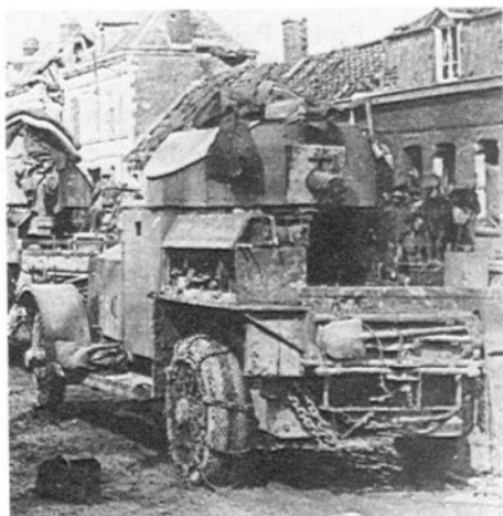
ABOVE LEFT: Rolls-Royce armoured cars at Arras in April 1917. The chains on the rear wheels gave them better grip, but conditions on the Western Front favoured the tank, introduced in September 1916.
