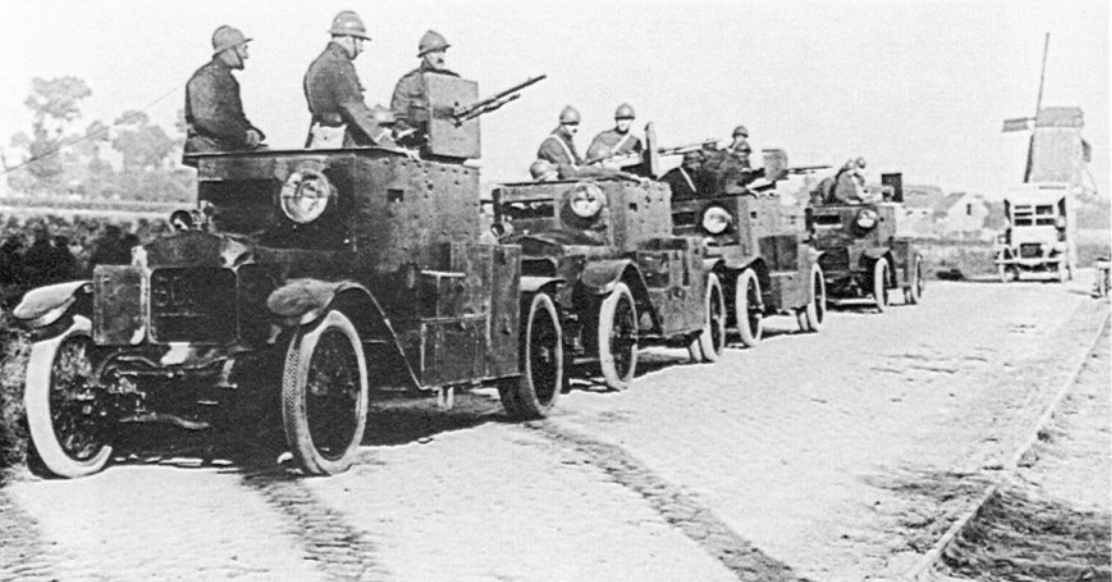
Belgian Army Minerva armoured cars at Houthem, near Ypres, in September 1917. They all have 8 mm machine-guns.
