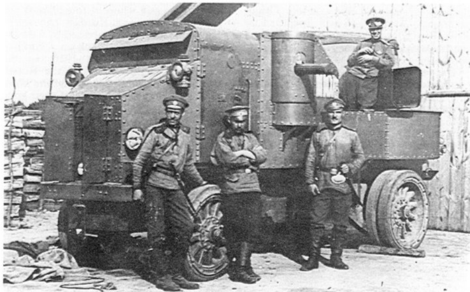
BELOW: The massive Putilov-Garford was one of the most powerfully armed armored cars of the First World War. One of the eight crewmen is leaning against the steel channels shielding the 76 mm gun, his arms around the co-axial Maxim machine-gun. Another crewman is standing beneath one of the sponson-mounted machine-guns.
