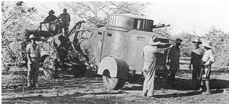
The Italian Army used the 1917-model Lancia IZ for many years. It fought in the Civil War in Spain and was still in use during the Second World War. The armoured car had a high ground clearance and could cross rough terrain, but this Lancia seen in East Africa has smashed a front axle.
